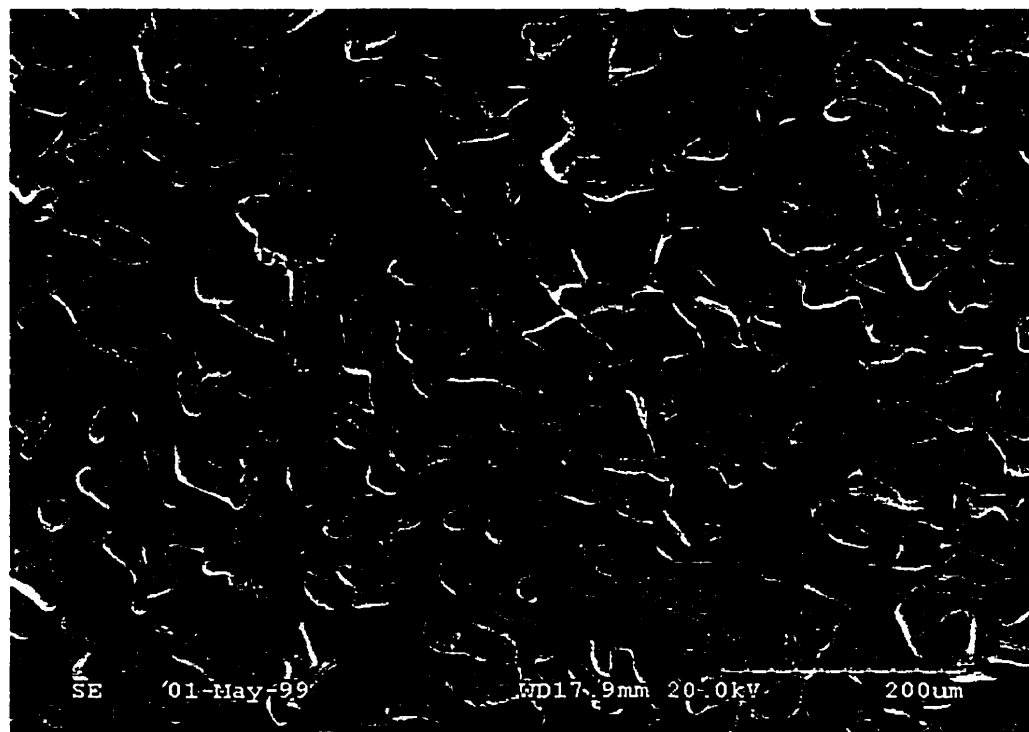
Figure 5.48: Higher magnification of Figure 5.47, showing a central region of large interconnected pores surrounded by smaller less interconnected pores.
