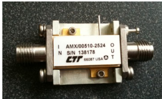
Figure 3.4. The low-noise amplifier (LNA).
