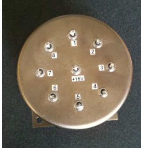
Figure 3.3. The 8-port Dow-Key Microwave switch.
