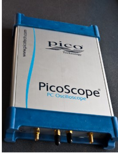
Figure 3.2. The PicoScope PC Oscilloscope suggested for the experimental set-up.
