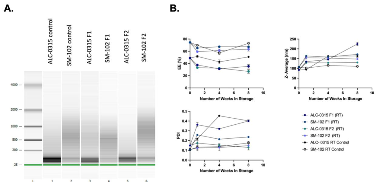
**Figure 3.3.** Stability Evaluation of mRNA-LNP samples stored at room temperature over the course of 2 months, with (A) demonstrating the mRNA integrity of the mRNA after 8 weeks and (B) demonstrating the evolution of the encapsulation efficiency (EE), the z-average and the PDI over the course of the storage duration. Error bars represent the standard deviation between measurements.
