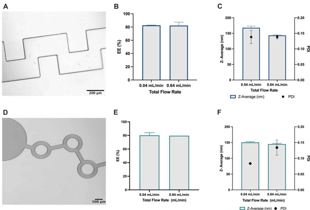
**Figure 2.7.** Summary of all critical quality attributes assessed demonstrating feasibility of the techniques. (A-C) illustrate the obstruction mixer and the quality attributes of the particles produced by it at a low (0.04 mL/min) and higher (0.64 mL/min) flow rate, (D-F) illustrate the ring micromixer and the quality attributes
