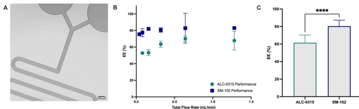
**Figure 2.2.** Demonstration of the Impact of Ionizable Lipid Choice on mRNA-LNP complexation in (A) microfluidic serpentine channels. (B) Results of encapsulation efficiency as a function of flow rate reveal
