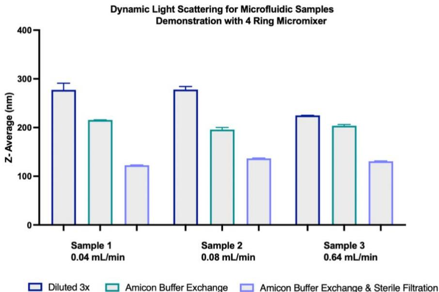
After Microfluidic Operation, to remove excess lipids and lipid aggregates prior to DLS analysis, it was recommended to perform a buffer exchange using Amicon MWCO 100kDa tubes and sterile filtering the LNPs produced in order to accurately measure the size of the mRNA-LNPs. We demonstrate here the change in size observed as we perform each step of this process.
