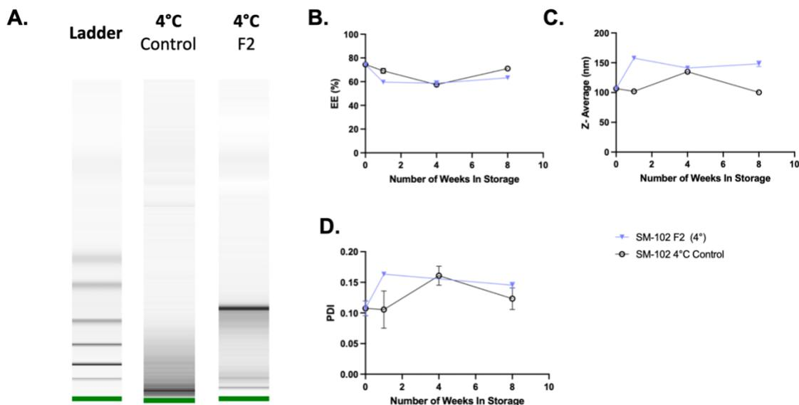
**Figure 3.5.** Stability Evaluation of SM-102 mRNA-LNP samples stored at 4°C over the course of 2 months, with (A) demonstrating the mRNA integrity of the mRNA after 8 weeks and (B) demonstrating the change of the encapsulation efficiency (EE), (C) the z-average and the (D) PDI over the course of the storage duration. Error bars represent the standard deviation between measurements. Controls represent samples in Tris buffer without additional excipients.
