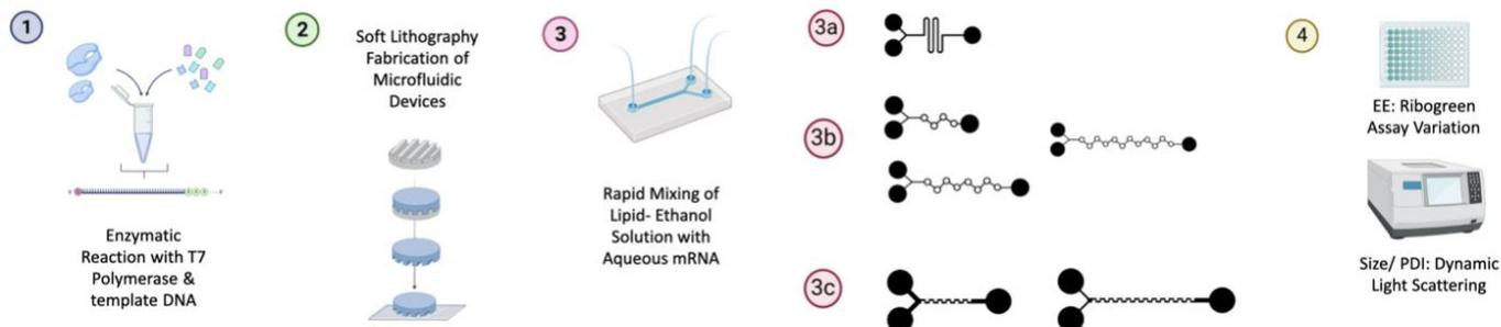
**Figure 2.1.** Overall Pipeline for Production and Characterization of mRNA-LNPs for the study. (3a), (3b) and (3c) illustrate the evaluated microfluidic device designs for the encapsulation of mRNA into LNPs.
