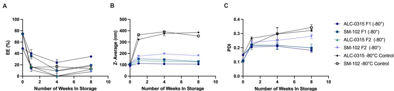
**Figure 3.7.** Change in the (A) encapsulation efficiency (EE), (B) size and (C) polydispersity index (PDI) of nLuciferase encoding mRNA-LNPs over the course of two months at  $-80^{\circ}\text{C}$ . Error bars represent the standard deviation between duplicate measurements.
