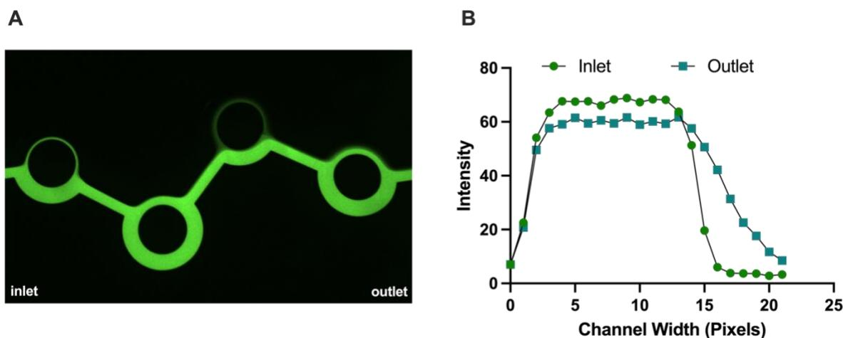
**Figure 2.3.** (A) Fluorescent imaging of the flow of acetate buffer and absolute ethanol streams at a total flow rate of 0.4mL/min (FRR=3) in a 4 ring micromixer. (B) Intensity profiles from the inlet and outlet of the microfluidic channels.
