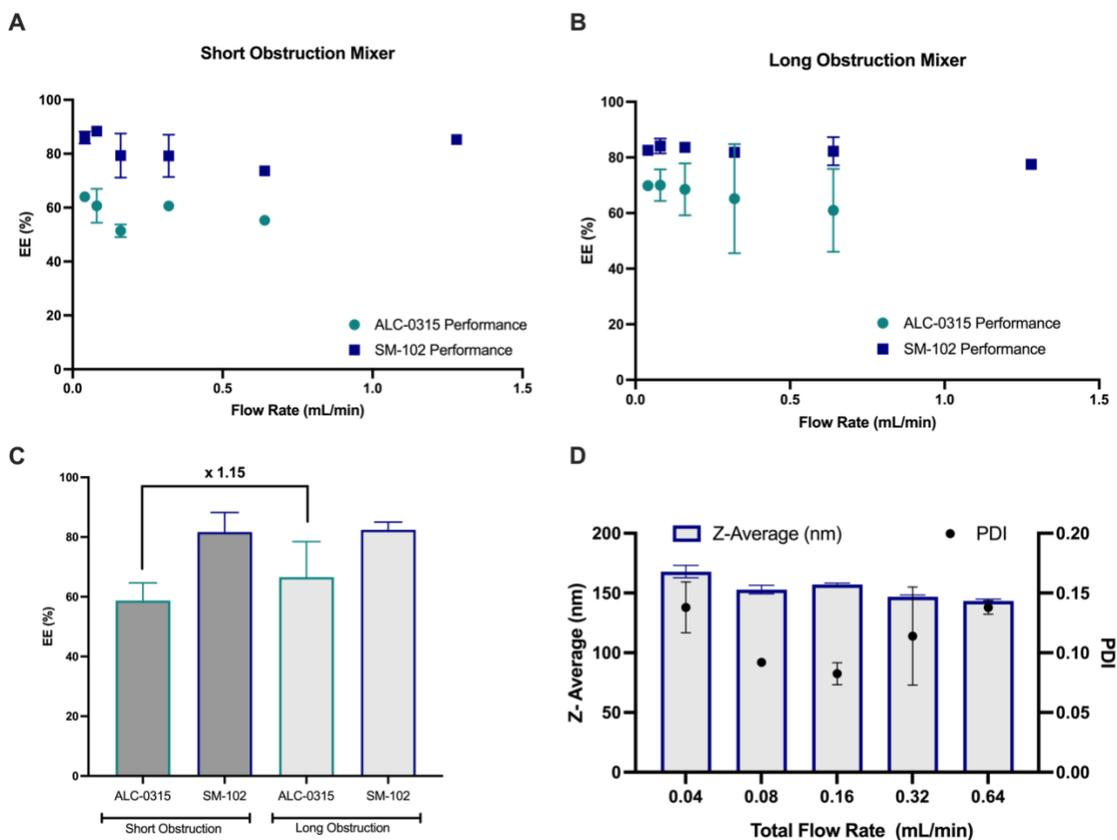
**Figure 2.6.** (A) Encapsulation Efficiency as a function of flow rate for short (12 obstructions) mixer and (B) long (24 obstructions) mixer, (C) Mean encapsulation efficiencies across all flow rates assessed classified by ionizable lipid and type of mixer used and (D) Sizes and PDI of ALC-0315 mRNA-LNPs produced using the long (24 obstructions) mixer.
