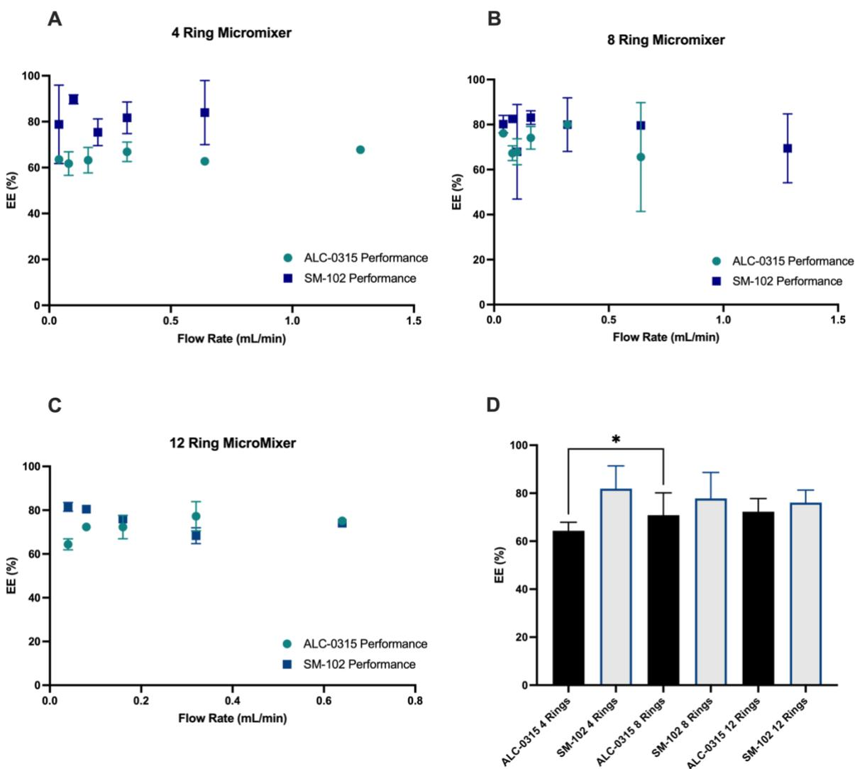
**Figure 2.4.** Encapsulation efficiency achieved as a function of flow rate in (A) 4 ring micromixer (B) 8 ring micromixers and (C) 12 ring micromixers (Error bars represent standard deviation between duplicate
