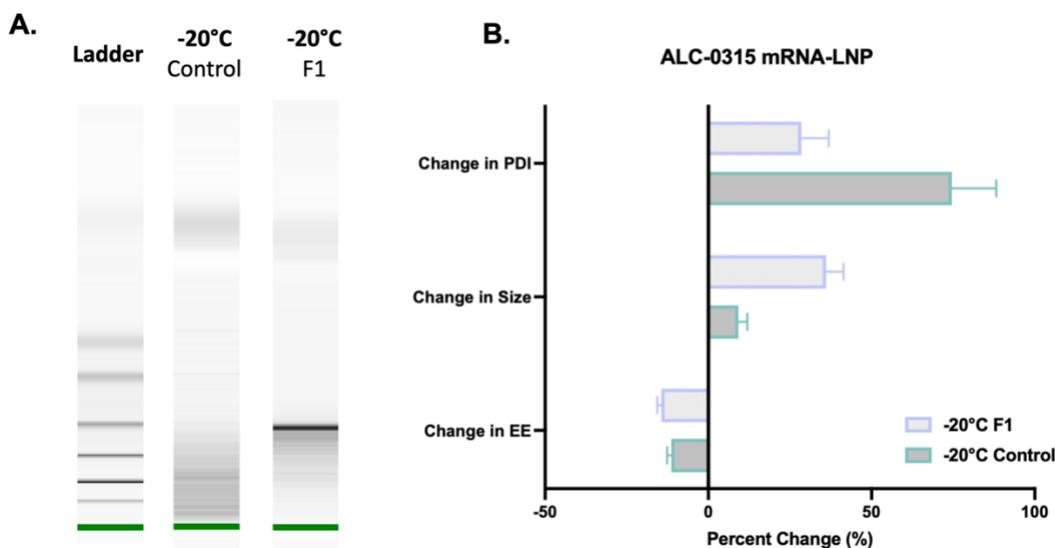
**Figure 3.6.** Stability Evaluation of ALC-0315 mRNA-LNP samples stored at  $-20^{\circ}\text{C}$  over the course of 2 months, with (A) demonstrating the mRNA integrity of the mRNA after 8 weeks and (B) demonstrating the percent change of the encapsulation efficiency (EE), the size (z-average) and the PDI over the course of the storage duration. Error bars represent the standard deviation between measurements
