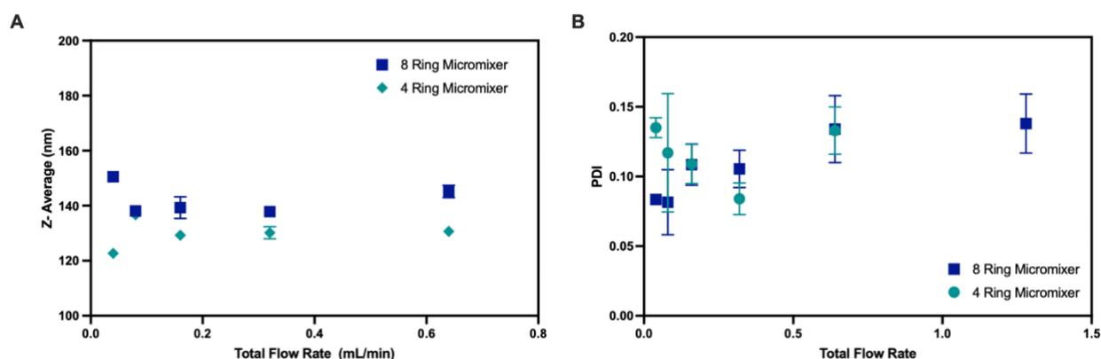
**Figure 2.5.** (A) Comparison of size measurements of ALC-0315 based mRNA-LNPs produced by 8 ring micromixers and 4 ring micromixers and (B) Comparison of their PDIs.
