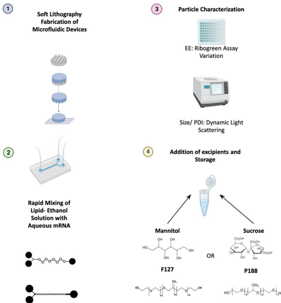
**Figure 9.1.** Schematic representing the entire process for mRNA loaded LNP manufacturing as optimized throughout the project.
