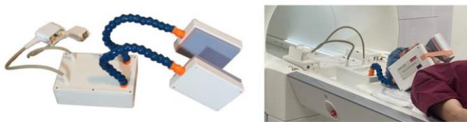
Fig. 5. The constructed 8-channel transmit-receive carotid coil
