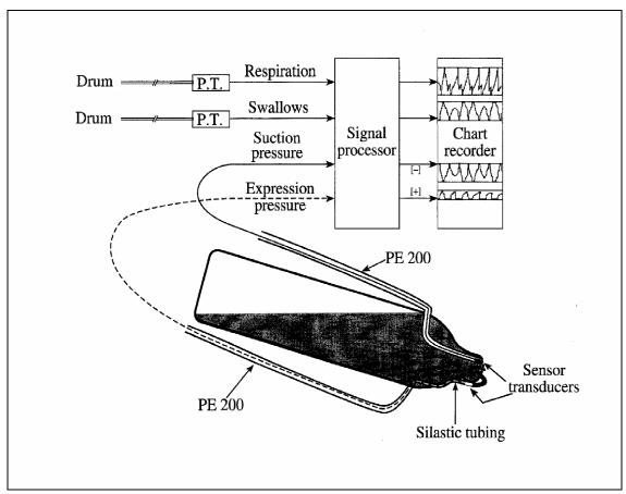
PT-pressure transducer, PE-polyethylene tubing
