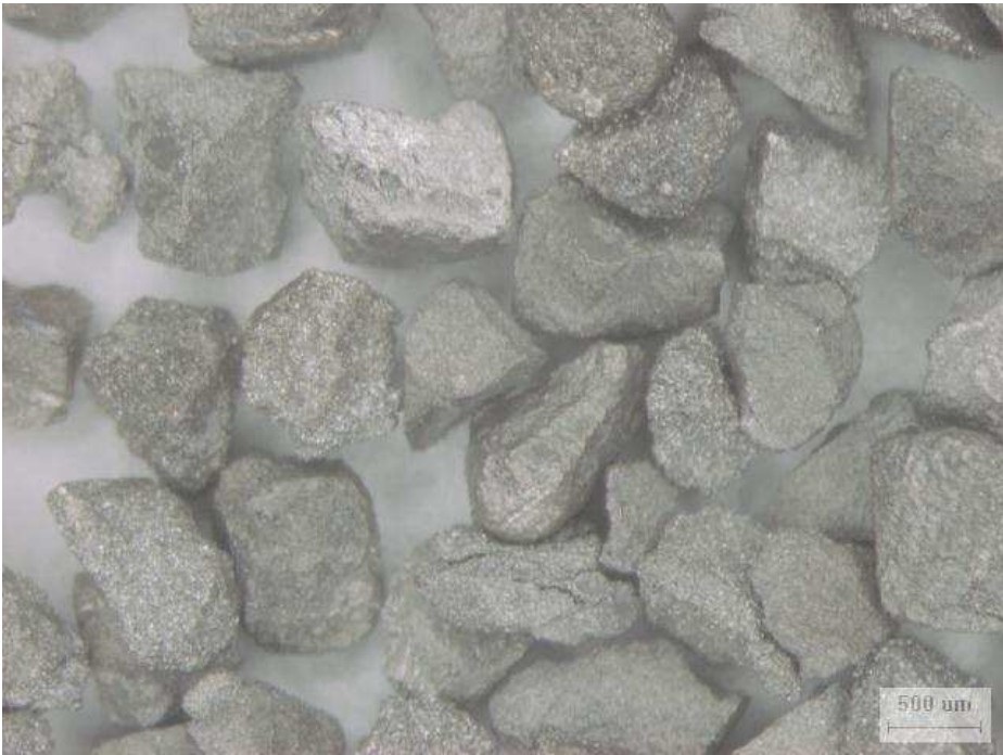
Figure 56: Tungsten particles (-850 + 600 μm)
