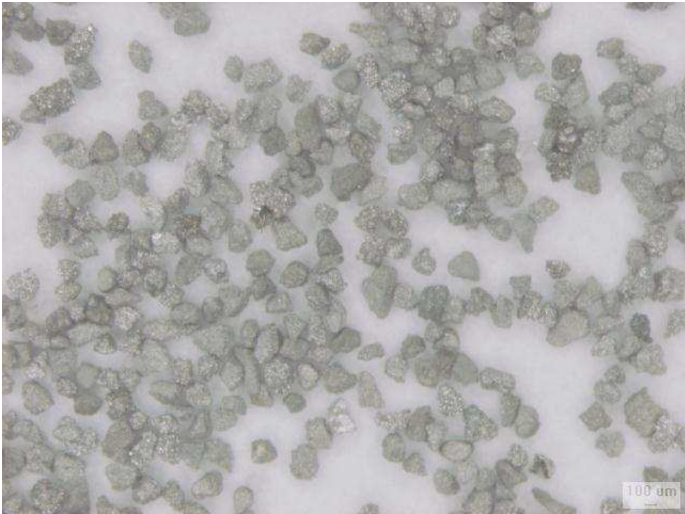
Figure 58: Tungsten particles (-212+ 150 µm)
