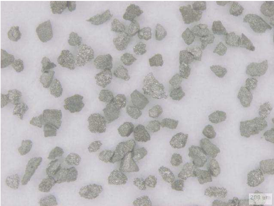
Figure 57: Tungsten particles (-300 + 212 μm)
