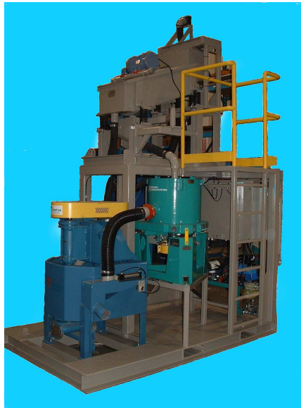
Figure 9: Pilot Knelson concentrator KC CD12 plant
