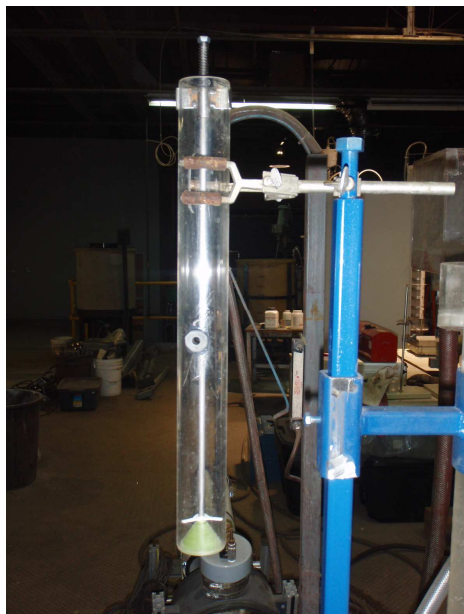
Figure 47: Feeding tube arrangement for introducing the dense particles
