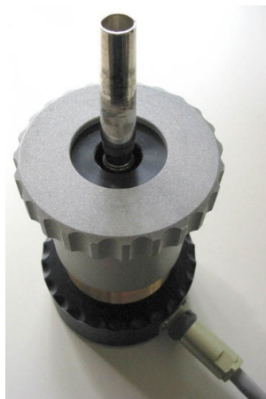
Figure 7 - The BIAS System, developed by the Institut für Wiener Klangstil, Vienna, Austria, is a commercially-available input impedance measurement system. A similar system, CapteurZ from the Centre de Transfert de Technologie du Mans, France, was used to gather the measurements in this document. Note the mouthpiece shank pointing upward from the top of the testing cylinder. 14
