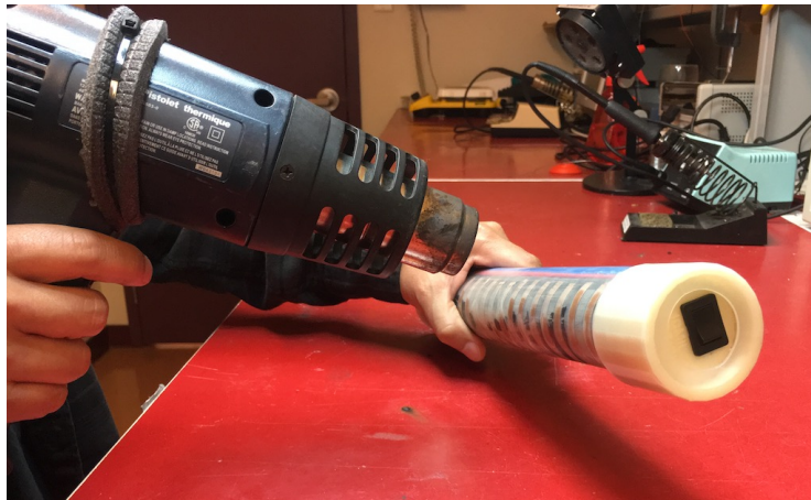
Figure 4.4 Finishing the construction of the Soprano 2GW-181 by wrapping it with transparent heat-shrink tube.
