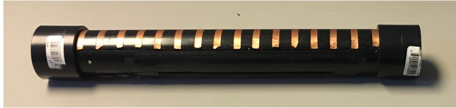
(b) The Soprano 2G fully assembled before being wrapped with heat-shrink tube.
