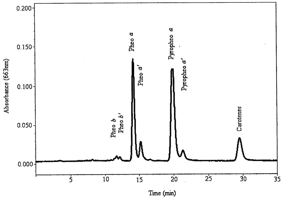
Figure 6. HPLC chromatogram of a crude commercial canola oil extract.
