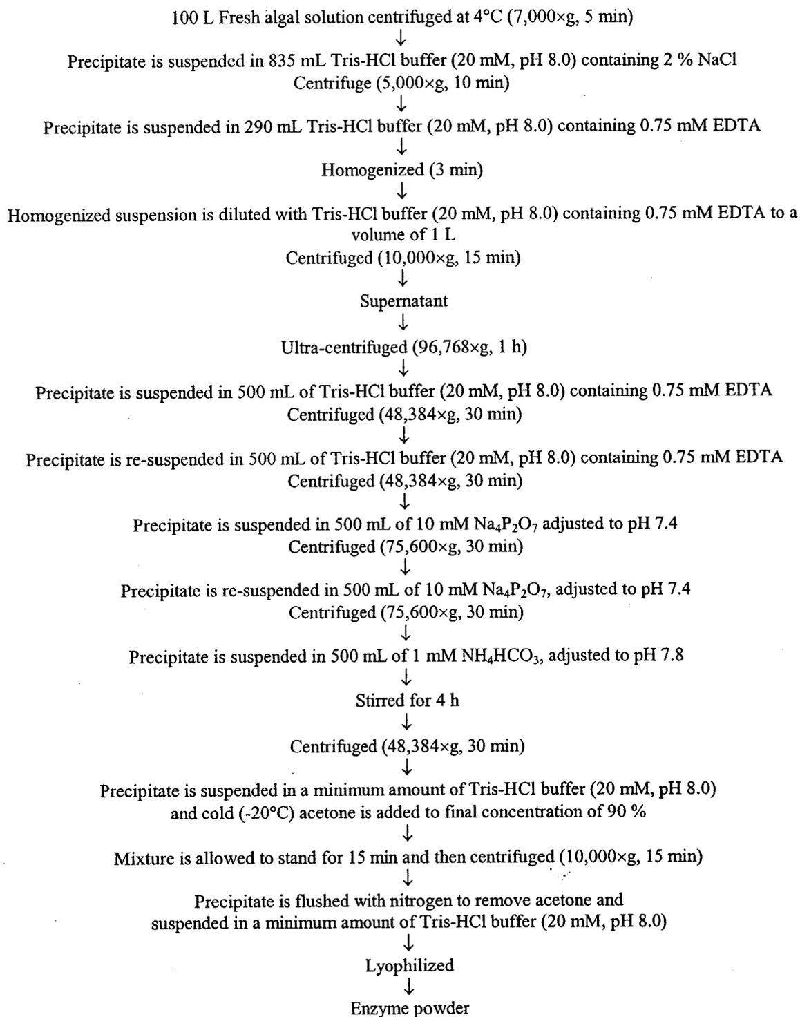
Figure 4. Schematic representation of the procedure for the partial purification of the chlorophyllase extract from the alga *P. tricornutum*.
