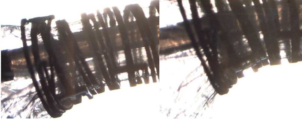
Figure 3.23: Struts at the extremities intertwine upon expansion
