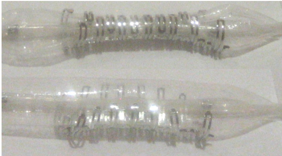
Figure 3.36: Expansion of the generation 3 stent on a 5mm balloon
