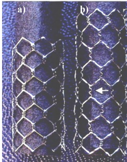
Figure 1.15: Genesis stent a) undeployed, b) deployed; note the elongated hinges (white arrow). From [32]
