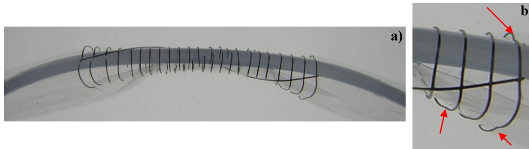
Figure 3.9: Helical stent deployed a) at 5mm b) Red arrows show hinge points along ribs
