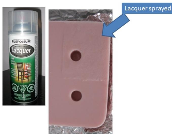
Fig. 3.6 – Coating Sil940 Substrate with Lacquer
