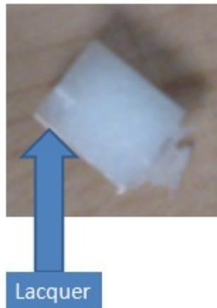
Fig. 4.17 – Scaffold Prepared in Lacquer Coated Sil940 Mold
