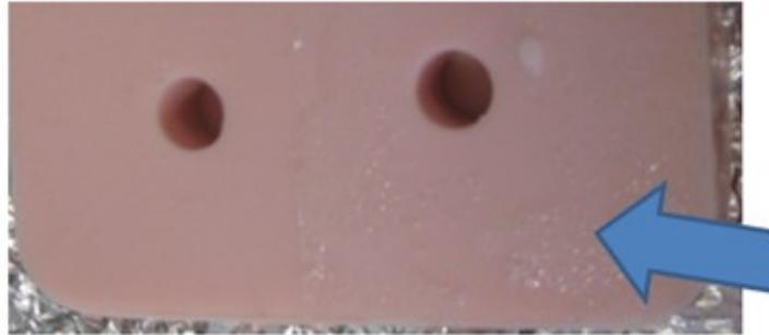
Fig. 4.18 – Deteriorated Lacquer Coating on Sil940 Mold
