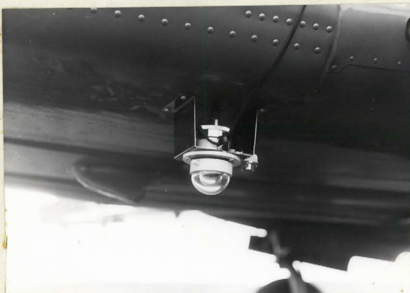
Photograph E: The mounting of the downfacing solarimeter on the Piper "Apache".
