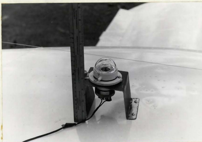
Photograph C: The mounting of the upfacing solarimeter. The same method was used on both aircraft.
