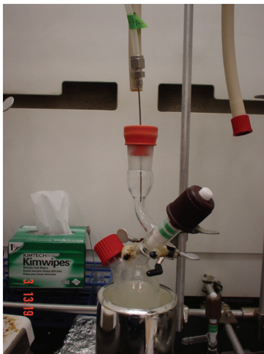
Figure 2.5 Transfer of 1,3-butadiene from gas cylinder into cylindrical flask at -78^{\circ}\text{C}
