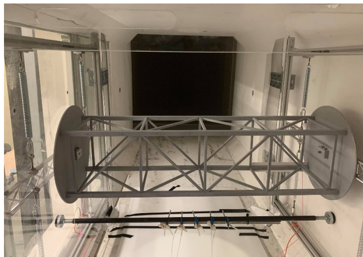
Figure 5-1 Truss specimen in TMU Wind Tunnel
