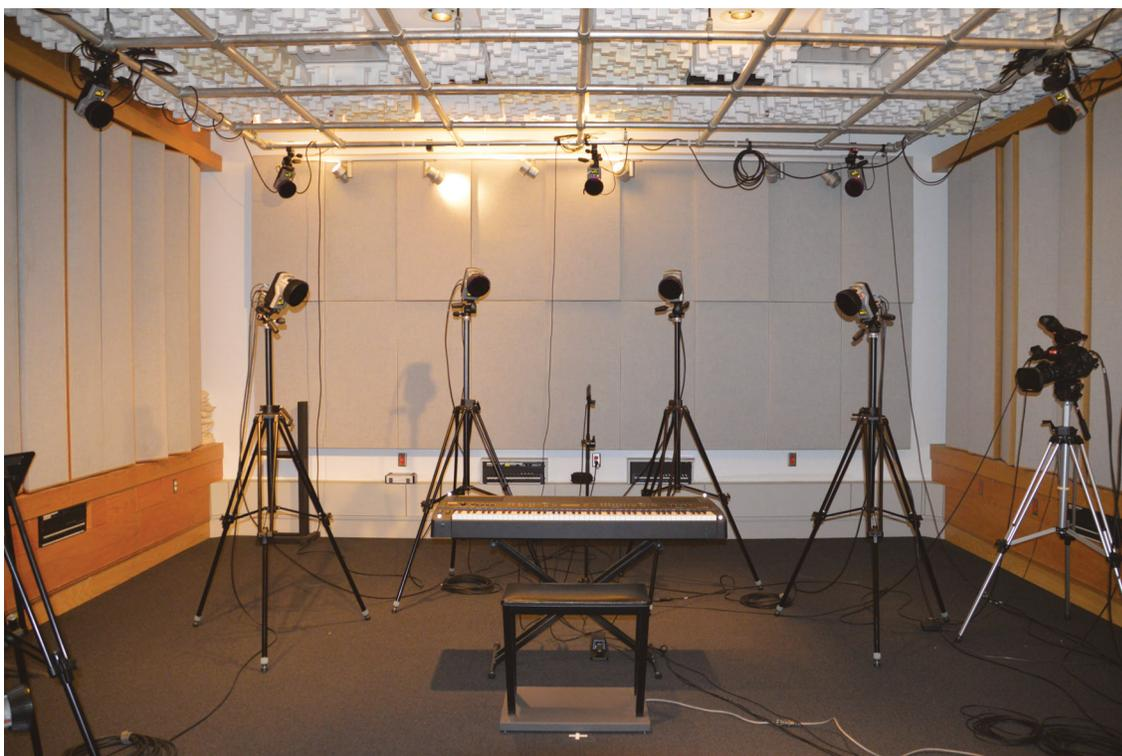
**Fig. B.2** Laboratory setup. Motion capture cameras, MIDI keyboard, force plate, video and audio recording are visible.
