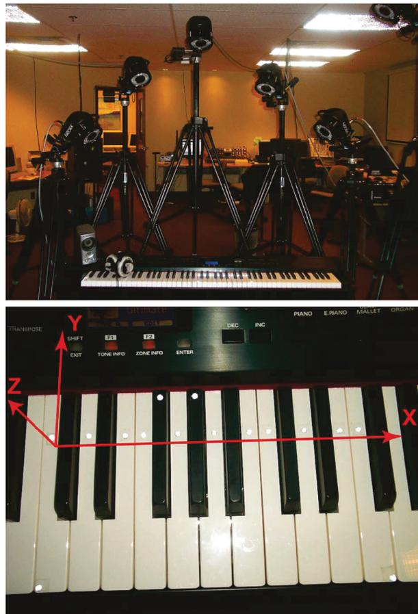
**Fig. 2.3** Motion capture setup and marker placement on the keyboard. Fifteen markers were placed on the piano keyboard and six infrared cameras were used. Figure from Goebel, W. and Palmer, C. "Temporal Control and Hand Movement Efficiency in Skilled Music Performance" in PLoS ONE, vol. 8, 1, 2013 (c) 2013 Goebel and Palmer. (Used under the terms of the CC BY license).
