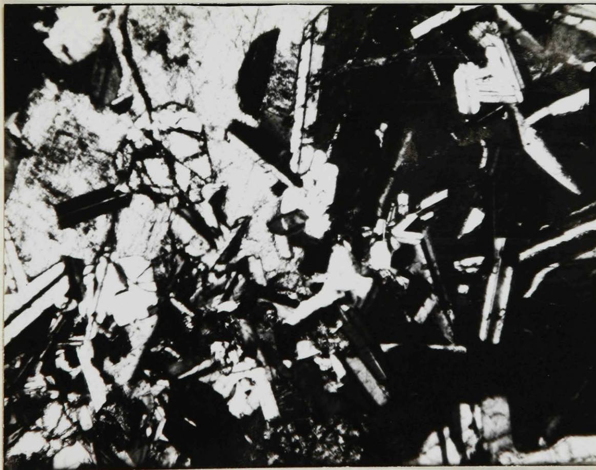
B. - Olivine diabase. Plagioclase laths included in two large crystals of augite. Note also small cracked olivine grain in northwest quadrangle. x45, polarized light.
