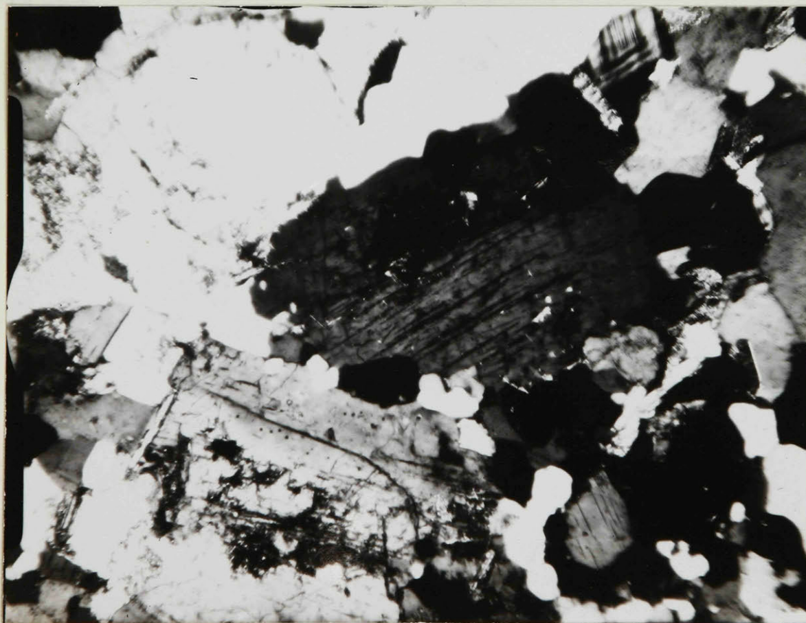
B. - Protoplastic texture in Maicasagi River Gneiss. Note the granulation between the two large oligoclase grains, in the center of the photograph. x45, ordinary light.
