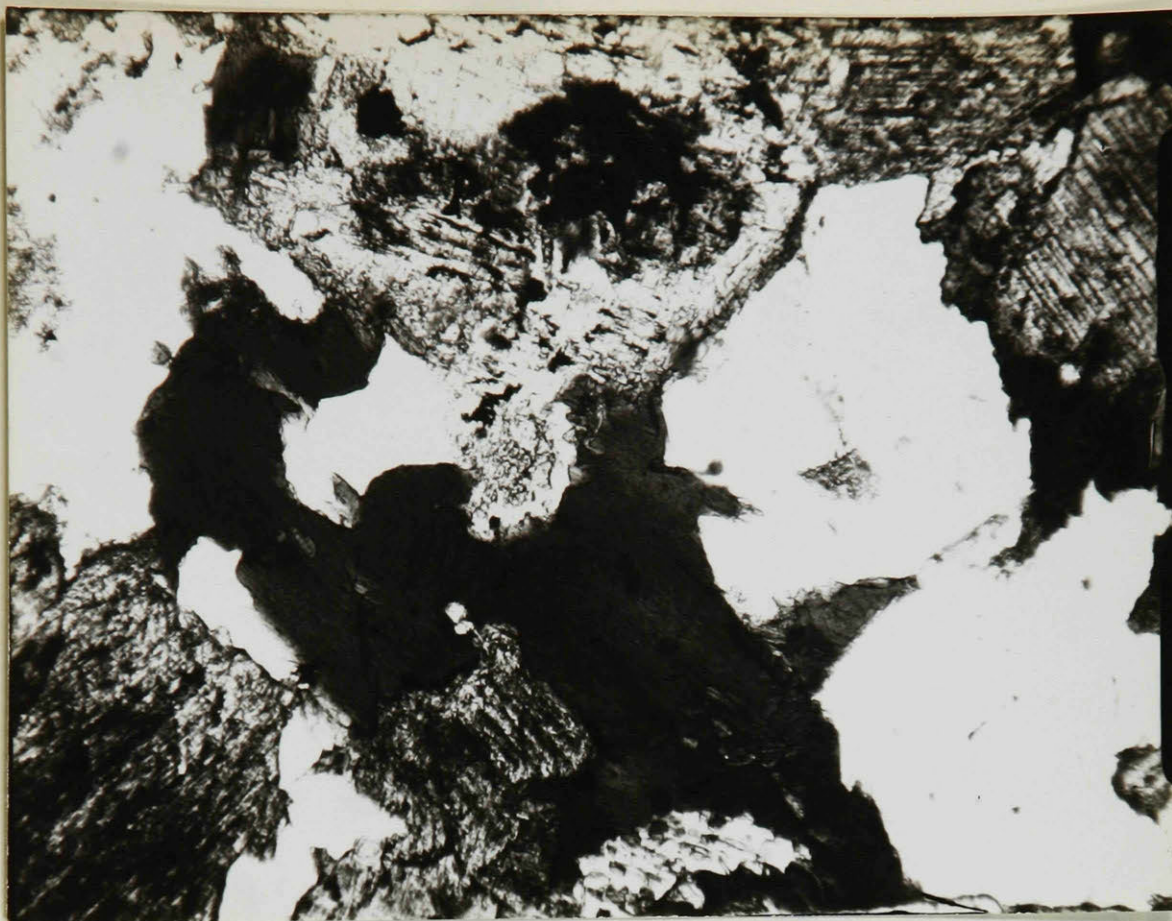
A. - Fresh dioritic facies of the Diorite-Syenite Complex. The large grain in the north central section is hypersthene with thick inclusions of iron oxides and a narrow rim of urallite at the periphery. The very dark mineral in the center is biotite which is associated with hypersthene and with diopside in the northeast and southwest corners. The colorless mineral is fresh andesine. x45, ordinary light.
