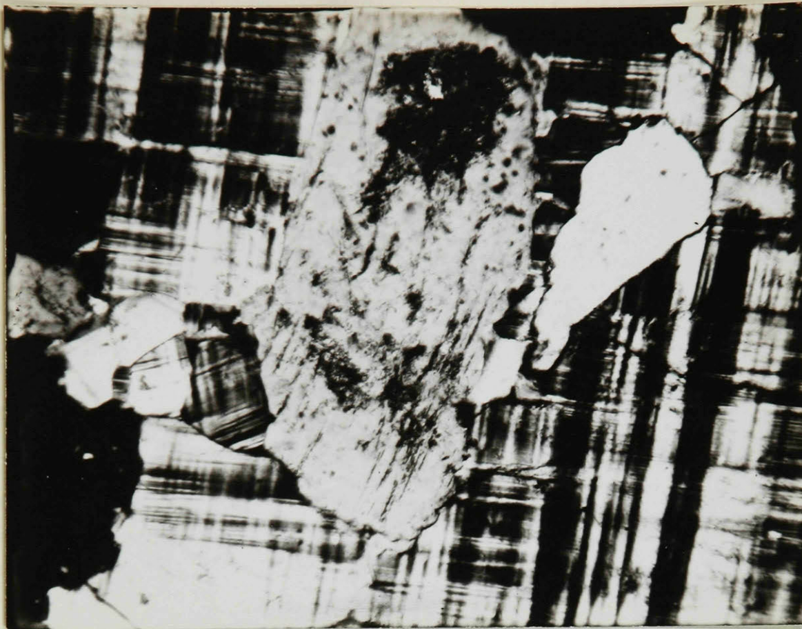
A. - Colorless quartz and slightly altered albite grain included in very large microcline crystal. x45, polarized light.
