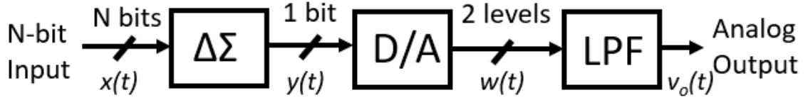
Fig.3.1 Typical structure of a \Delta\Sigma -based DAC
