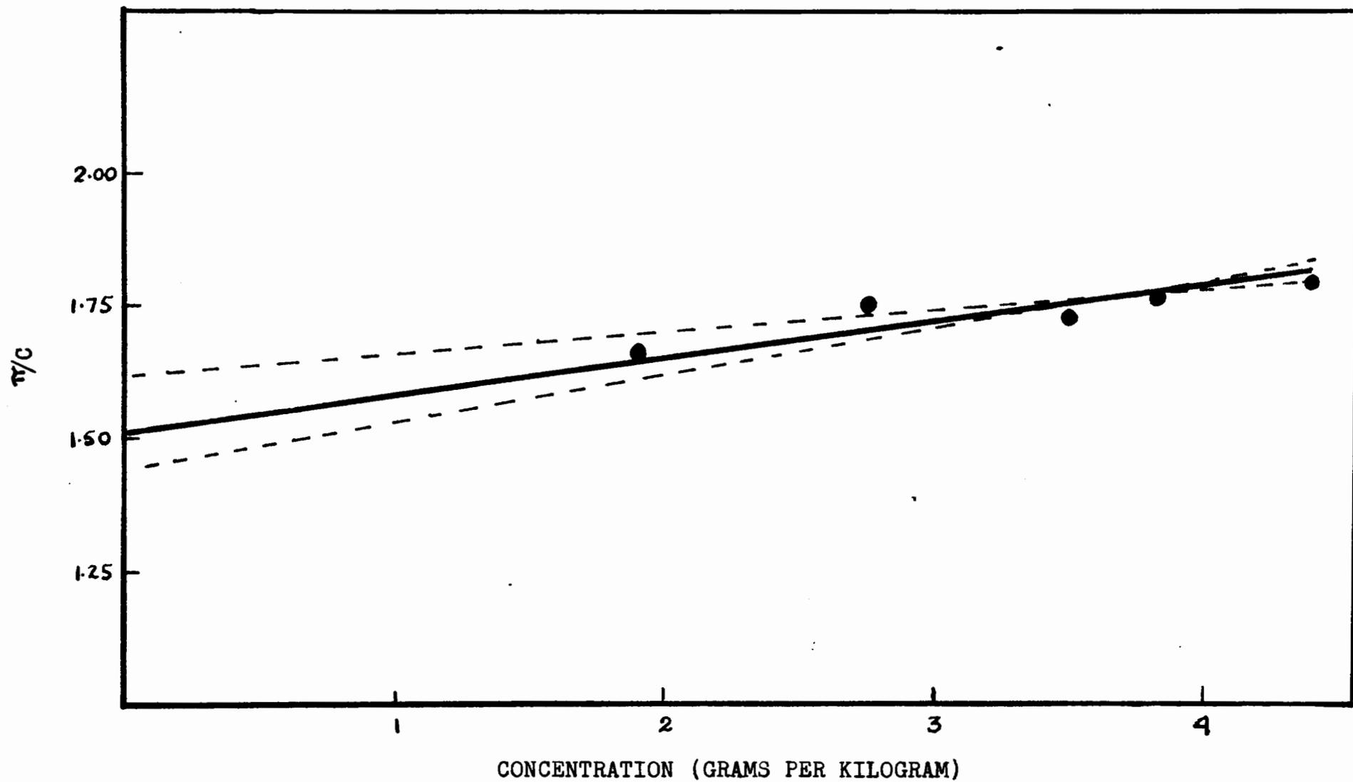
FIG. 4 Plot of Reduced Osmotic Pressure against Concentration for the Methylated Hemicellulose
