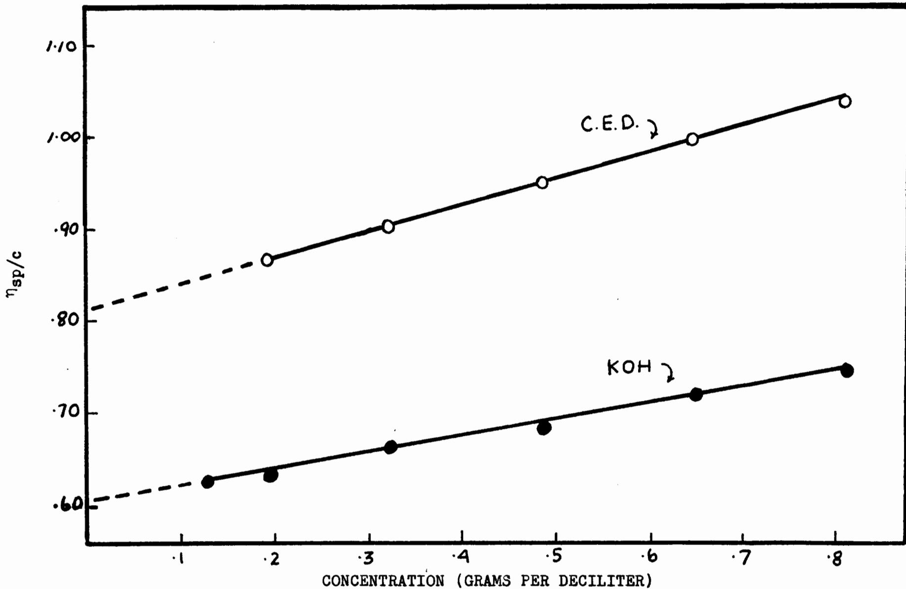
FIG. 3 Plot of Viscosity against Concentration for Milkweed Xylan in 10% (w/w) Potassium Hydroxide and M Cupriethylenediamine
