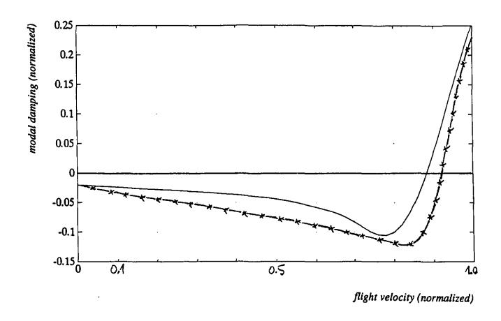
Normalized modal damping versus normalized flight velocity, for the unstable mode.
