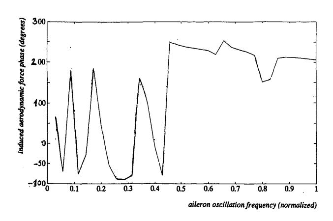
Figure 4.5  $Total\ aerodynamic\ force\ phase\ angle\ versus\ aileron\ oscillation\ frequency, for\ 2\ degrees\ aileron\ oscillation\ amplitude,\ and\ 1.43\ V$
