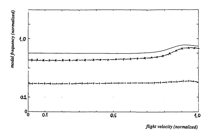
Normalized modal frequency versus normalized flight velocity, for the outboard bending mode.
