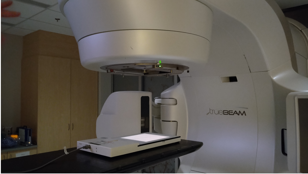
Figure 7-2: Setup for MapCHECK calibration and measurement.
