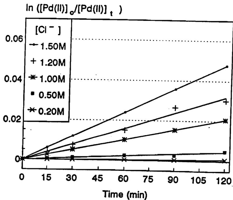
Figure 6.11 First order plots of Pd(II) stripping data at various  $Cl^-$  concentrations.
