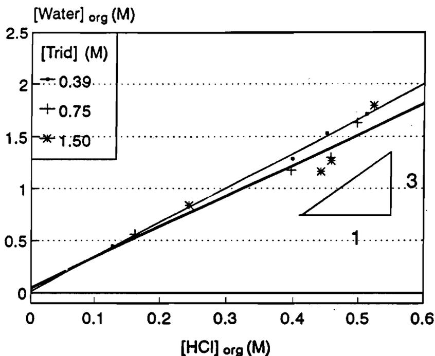
**Figure 3.15** Water and acid extracted in high acid region. Solvesso 150 solutions of  $[\text{TN 1911}]_{\text{org}} = 0.50\text{M}$ ,  $[\text{Tridecanol}]_{\text{org}} = 0.38, 0.75$  and  $1.50\text{M}$ .
