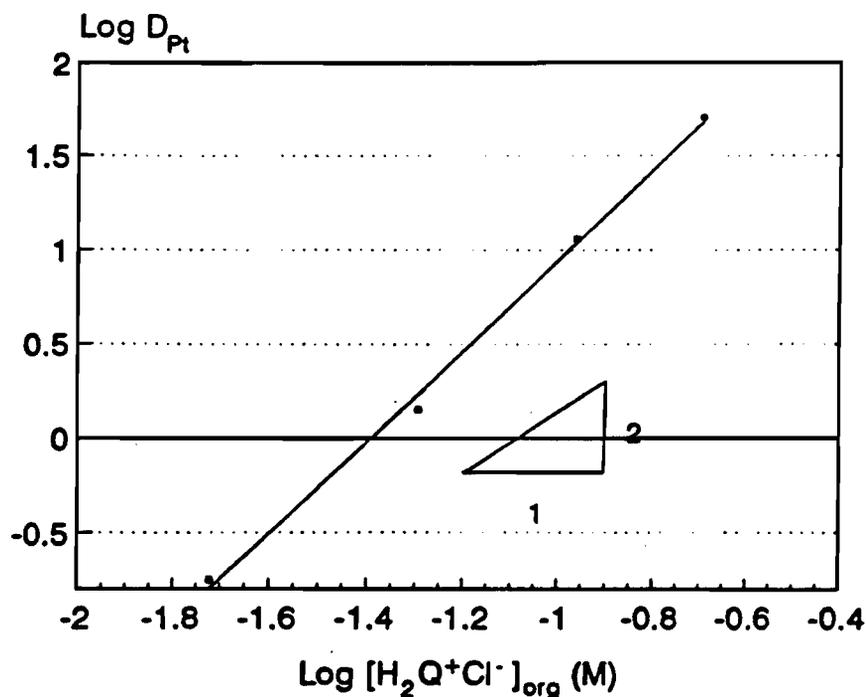
Figure 5.5 Log  $D_{Pt}$  as a function of log [protonated extractant]<sub>org</sub>.
