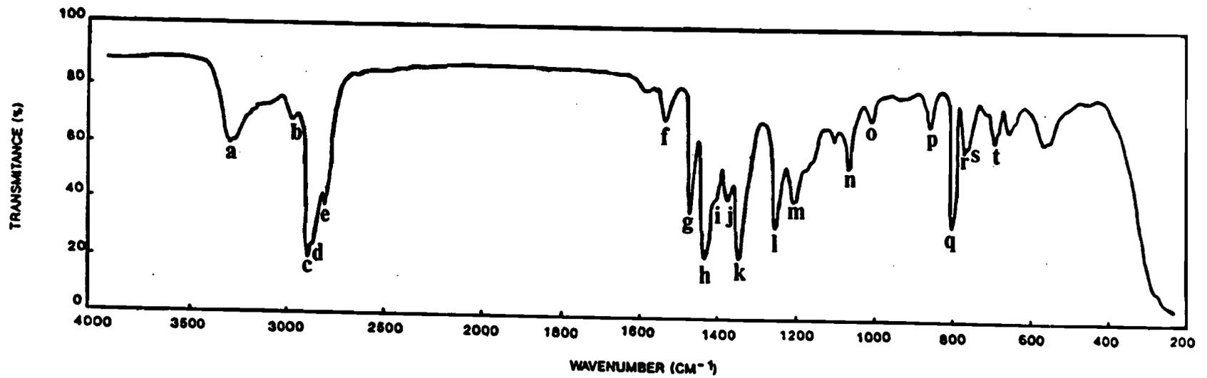
**Figure 3.3** Infrared spectrum of TN 1911 as a film on a NaCl cell.
