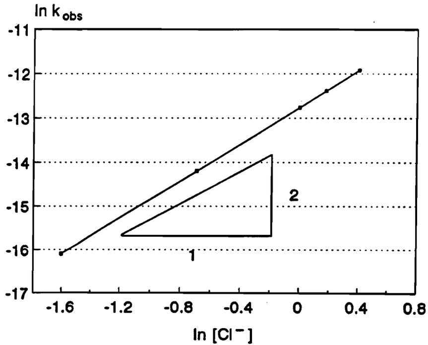
**Figure 6.13** Log-log plot of the observed stripping rate constant,  $\ln k_{obs}$ , versus  $\ln [Cl^-]$ .
