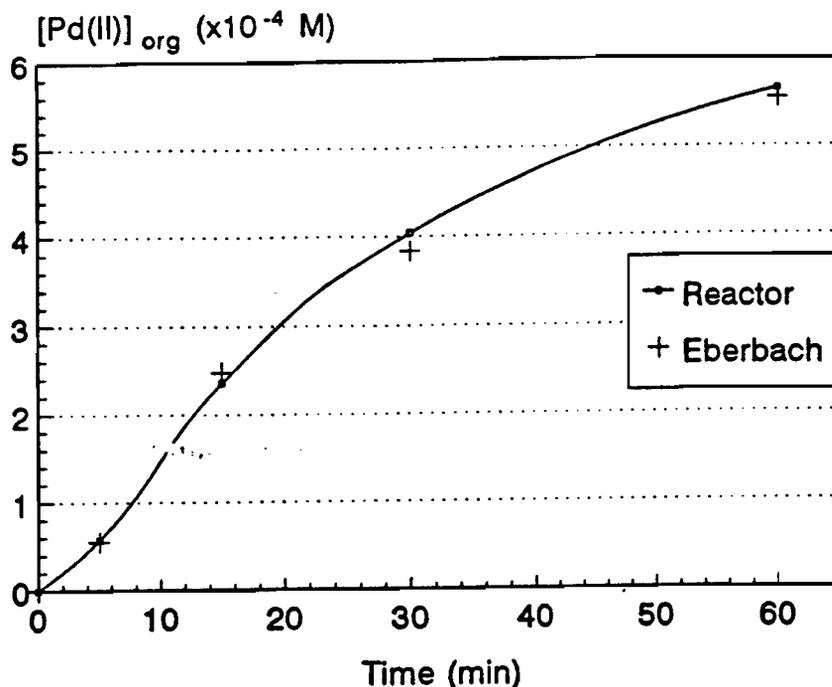
**Figure 6.1** Comparison of Pd(II) extraction kinetics measured with two different reactors, a box-type Eberbach shaker (280 osc/min) and a reactor at 350 rpm.
