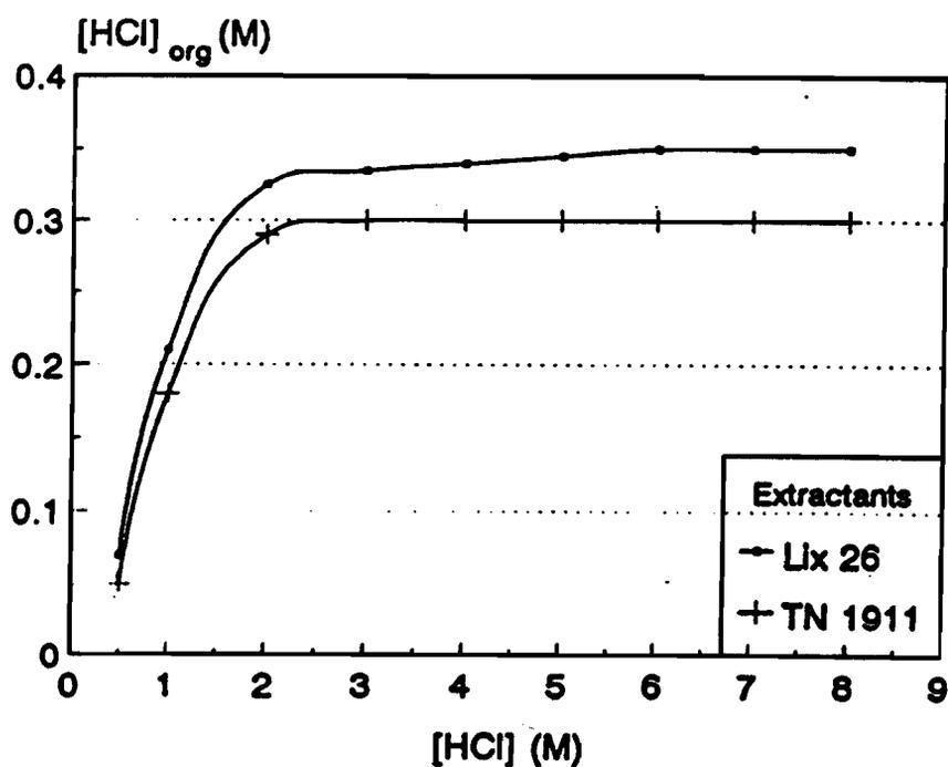
**Figure 3.7** HCl distribution in 0.3M TN 1911 and 0.3M Lix 26 in Solvesso 150 solutions at 25°C.
