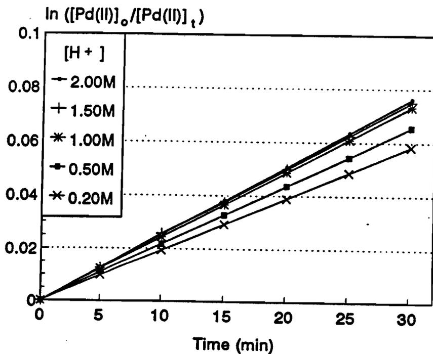
**Figure 6.3** First order plots of Pd(II) extraction data at various H<sup>+</sup> concentrations.
