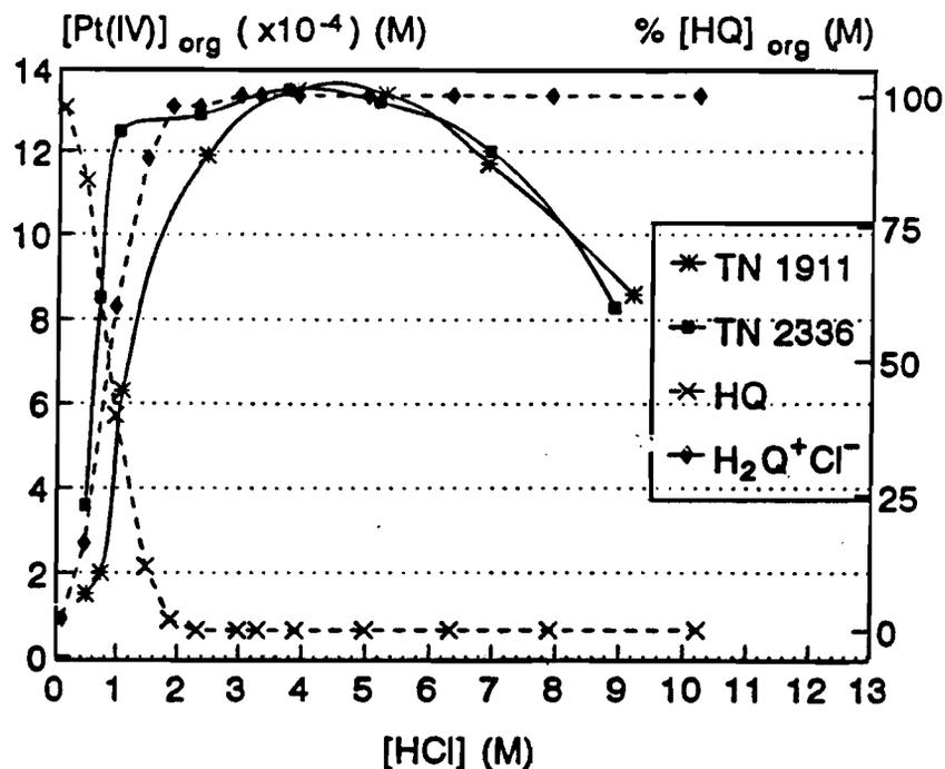
Figure 5.6 Platinum extraction and extractant speciation as a function of [HCl].
