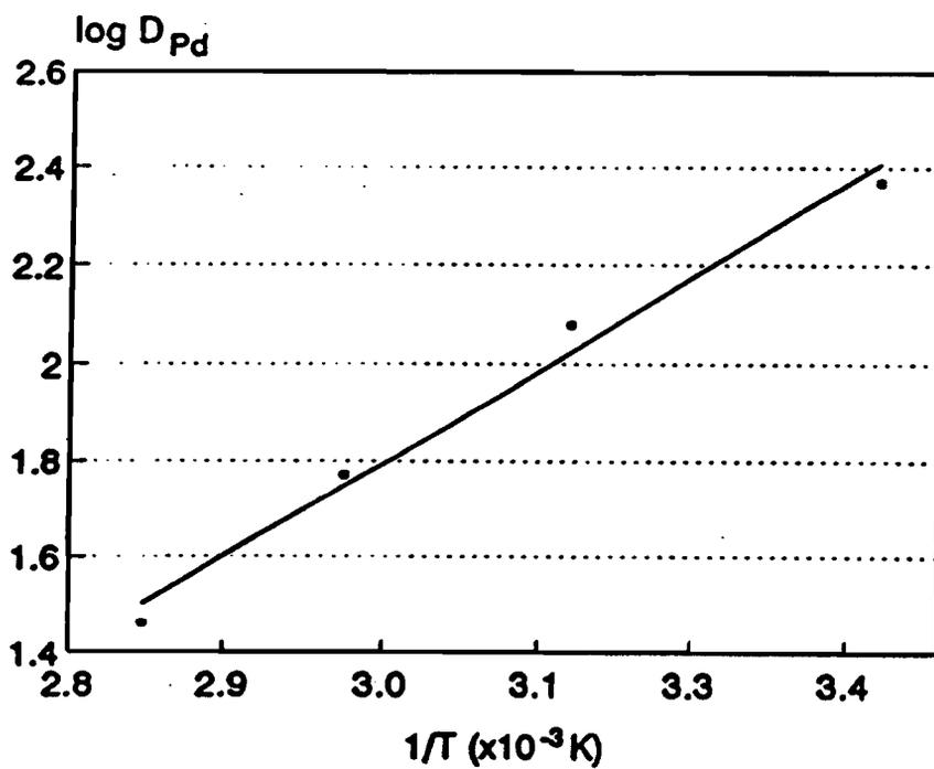
Figure 4.10 Van't Hoff plot for the system Pd(II)-TN 1911-HCl.
