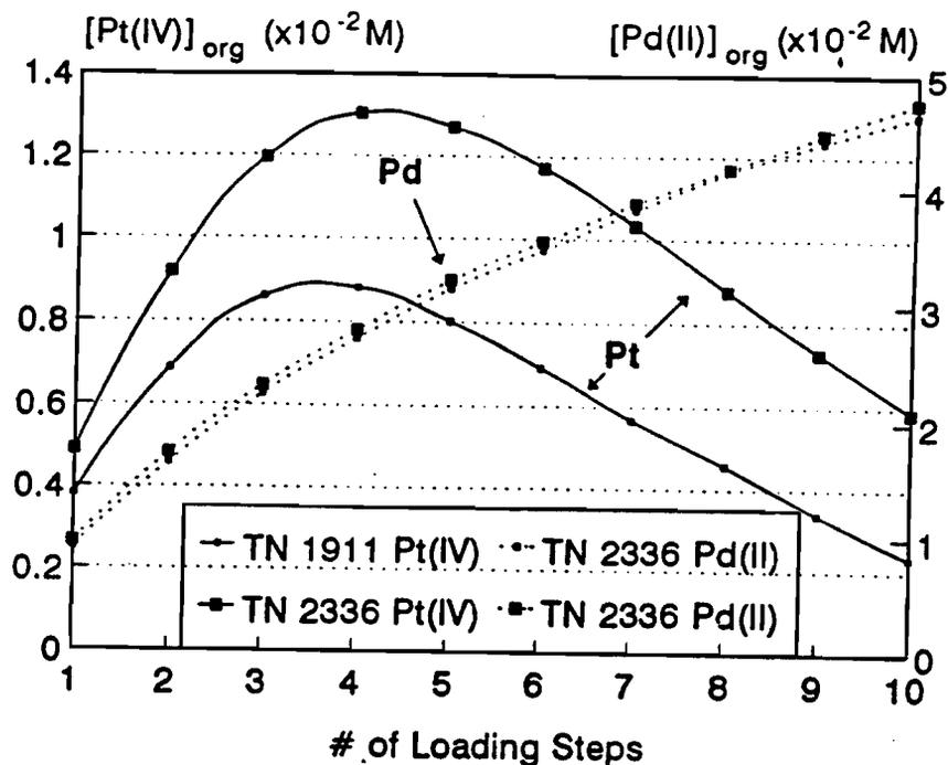
Figure 6.14 Pt(IV) and Pd(II) co-extraction from mixed metals solution as a function of number of loading stages.
