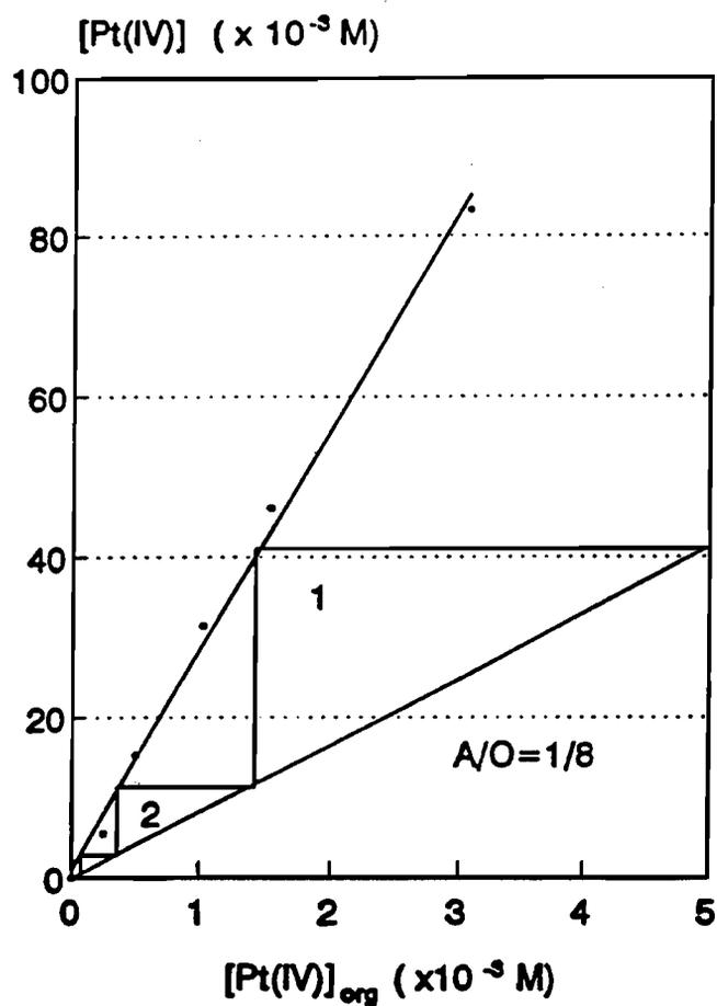
**Figure 5.13** Platinum stripping isotherm and McCabe-Thiele diagram.
