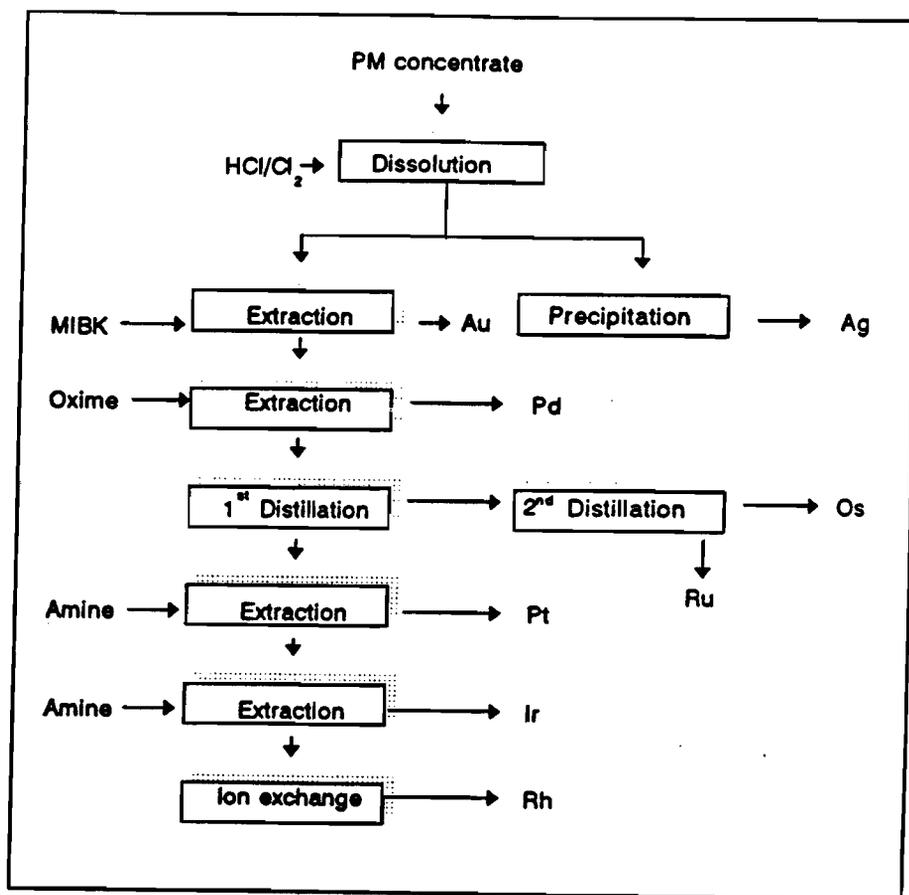
Figure 2.3 The Matthey Rustenburg Refiners flowsheet for the separation and recovery of PGM (5).
