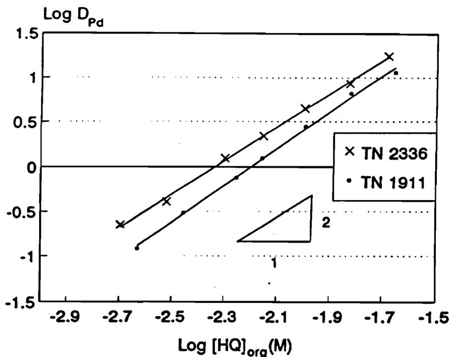
Figure 4.2 Log  $D_{Pd}$  as a function of log [Extractant] in  $CHCl_3$ .
