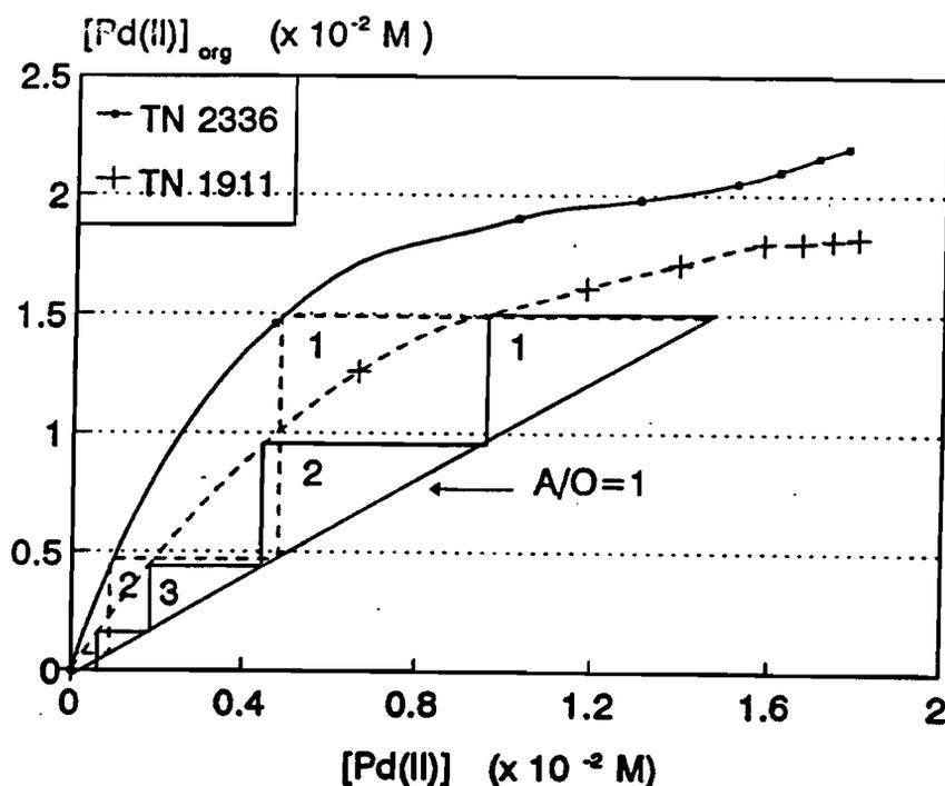
Figure 4.11 Palladium extraction isotherms and McCabe-Thiele diagram CT=15 minutes.
