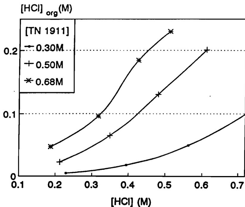
Figure 3.11 HCl extraction in low acid region  $[TN\ 1911]_{org} = 0.30, 0.50$  and  $0.68M$ . Solvesso 150 and Tridecanol were present.
