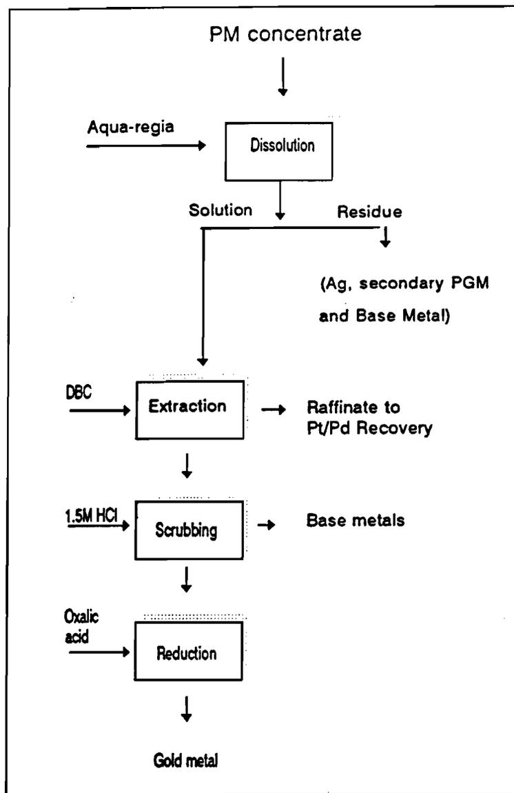
**Figure 2.1** The original INCO flowsheet for the separation and recovery of gold with SX (7).
