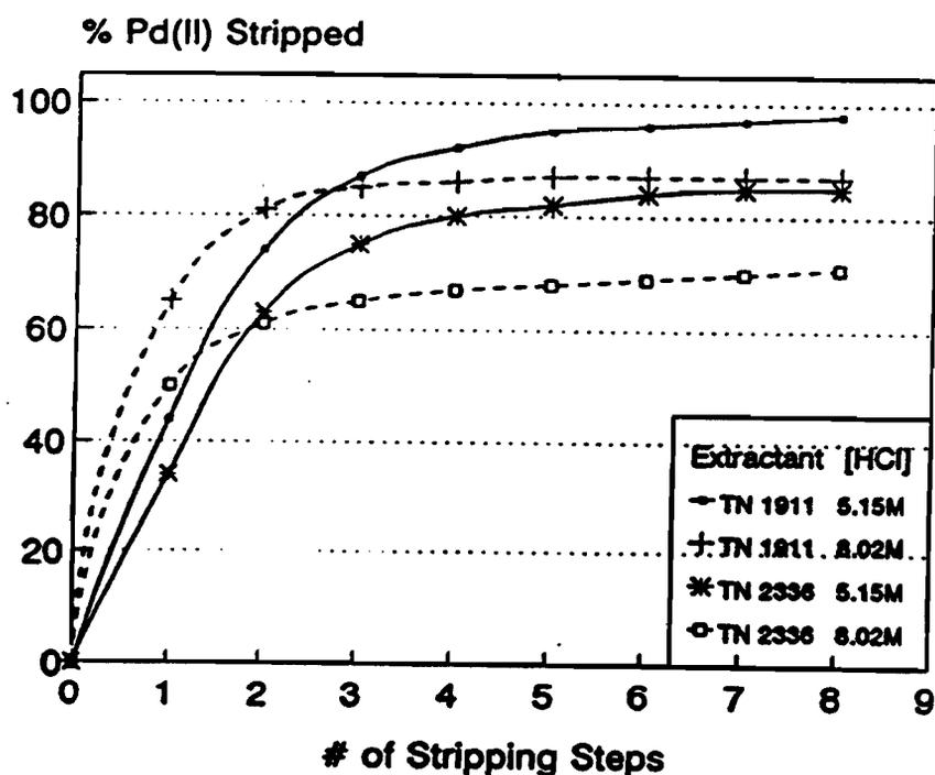
Figure 4.12 Stripping of palladium with 5.15 and 8.05M HCl as a function of consecutives stripping steps CT 3 min.
