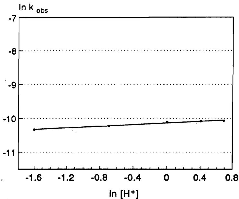
Figure 6.6 Log-log plot of the observed extraction rate constant,  $\ln k_{obs}$ , versus  $\ln [H^+]$ .
