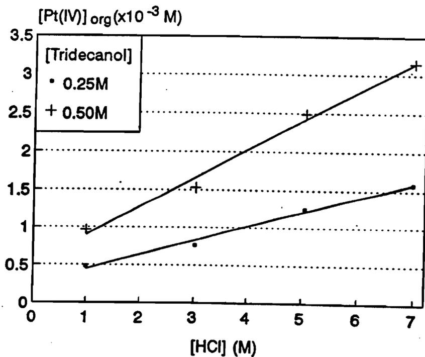
Figure C.2 Extraction of platinum by tridecanol as a function of  $[HCl]$ .
