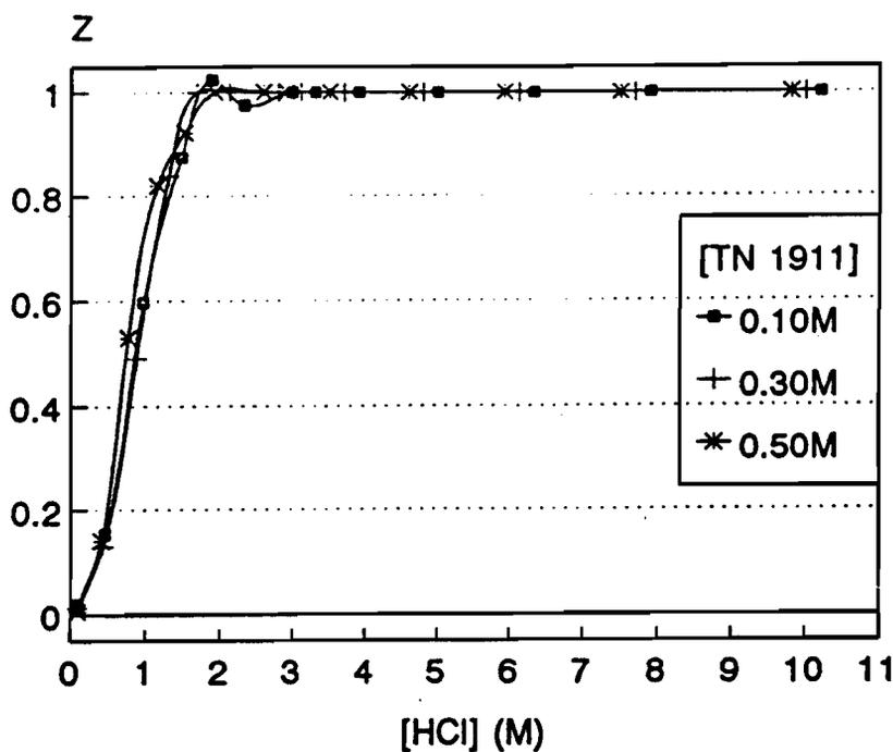
**Figure 3.9** Relation between distribution ratio of hydrochloric acid,  $Z$ , and HCl concentration in the aqueous phase.
