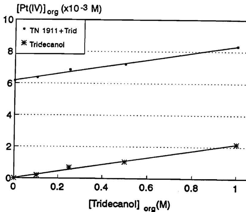
Figure C.3 Extraction of platinum as a function of  $[\text{Tridecanol}]_{\text{org}}$  with and without TN 1911.
