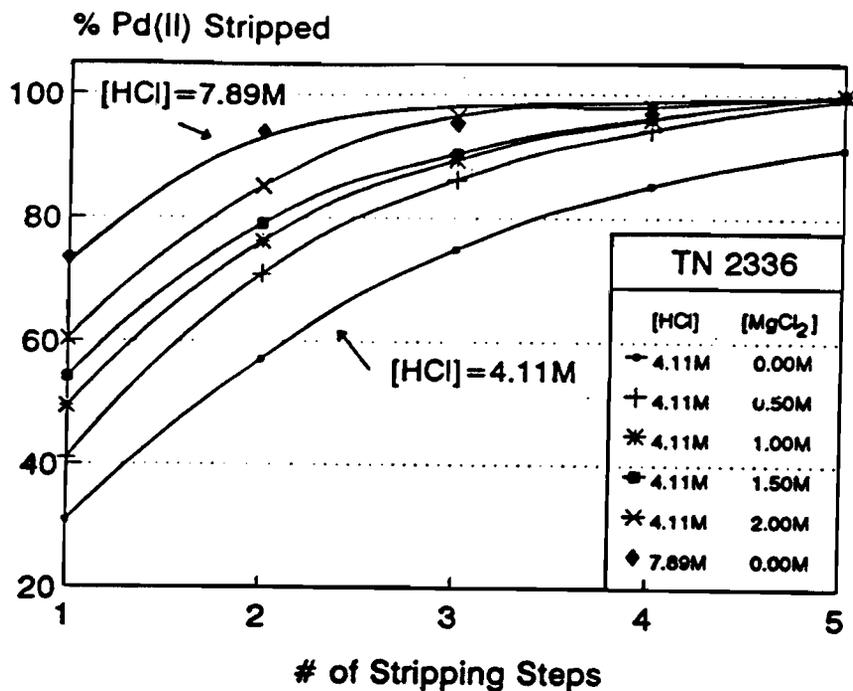
**Figure B.7** Stripping of palladium from loaded TN 2336 by 7.89M HCl and 4.11M HCl/0-2.00M MgCl<sub>2</sub> as a function of the number of consecutive stripping steps. CT 30 min.
