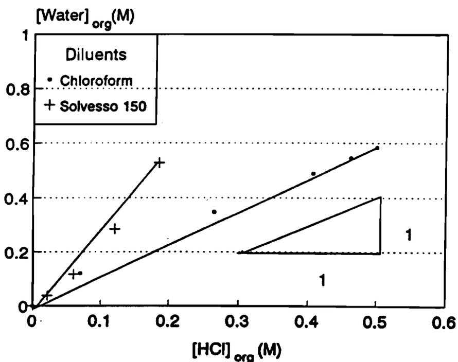
Figure 3.14 Water and acid extracted in low acid region.  $\text{CHCl}_3$  and Solvesso 150 solutions of TN 1911  $[\text{TN 1911}]_{\text{org}} = 0.50\text{M}$ .
