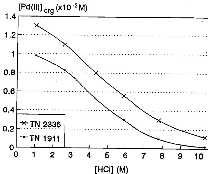
Figure 4.7 Extraction of palladium as a function of HCl concentration.
