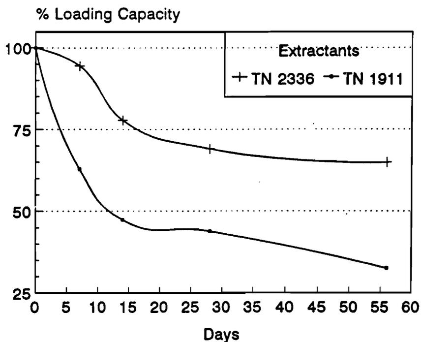
**Figure A.1** Long term chemical stability of 8-HQ extractants against HCl attack.
