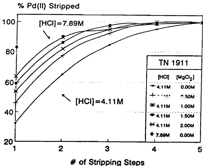
**Figure 4.13** Stripping of palladium by 7.89M HCl and 4.11M HCl/0-2.00M MgCl<sub>2</sub> as a function of the number of consecutive stripping steps CT 30 min.
