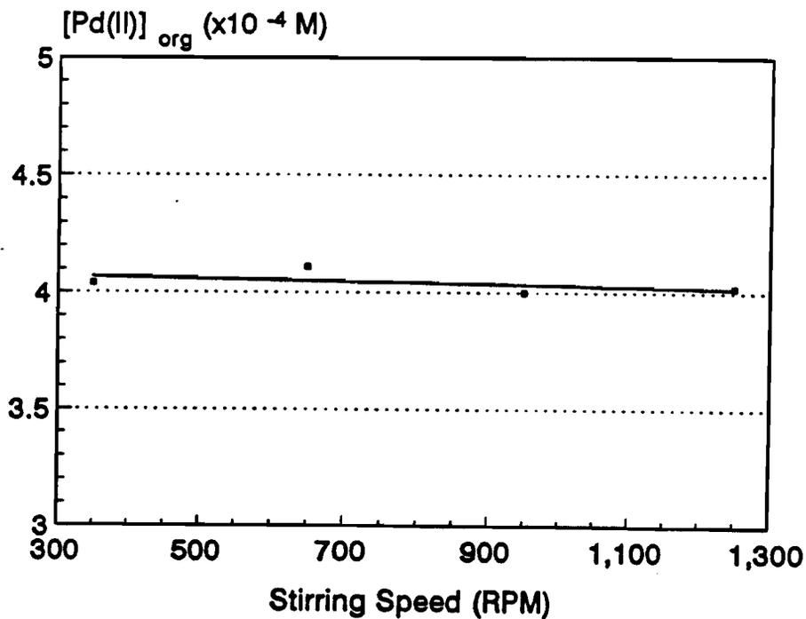
**Figure 6.2** The effect of stirring speed on the extraction level of Pd(II) after 30 min. mixing time.
