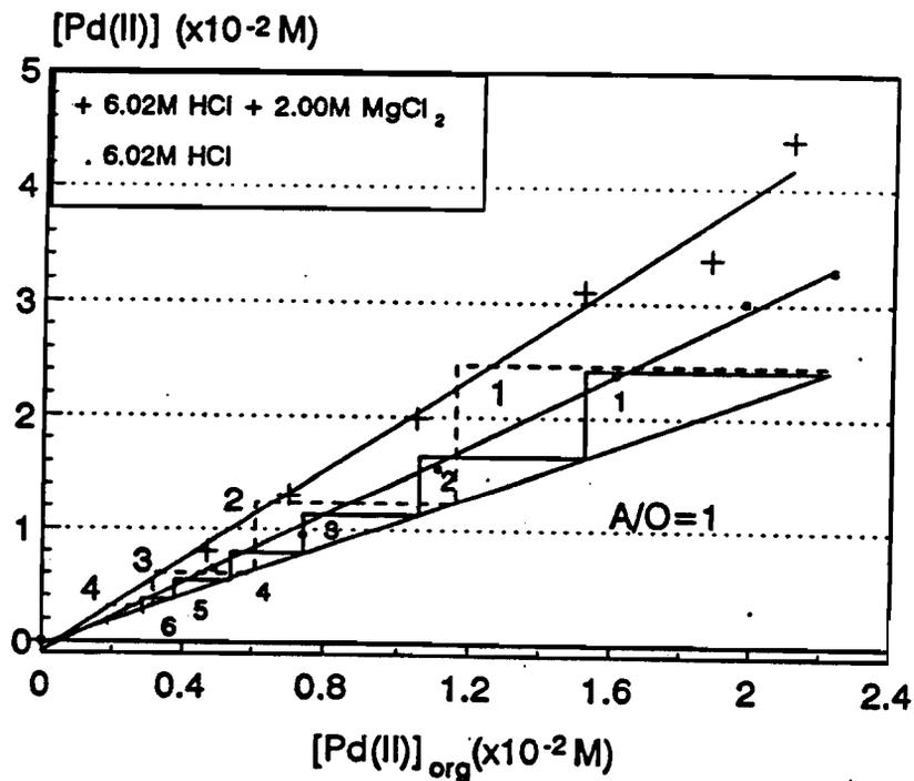
Figure B.5 Palladium stripping isotherms and McCabe-Thiele diagram; stripping agents 6.02M HCl and a mixture 6.02M HCl+2.00M MgCl<sub>2</sub>, CT 3 min.
