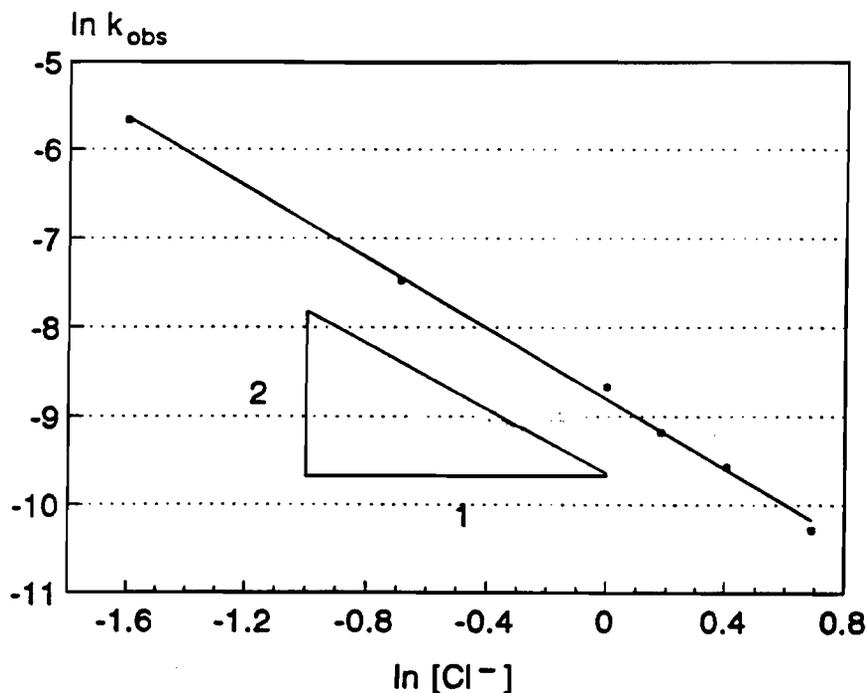
**Figure 6.8** Log-log plot of the observed extraction rate constant of Pd(II),  $\ln k_{\text{obs}}$ , versus  $\ln [\text{Cl}^-]$ .
