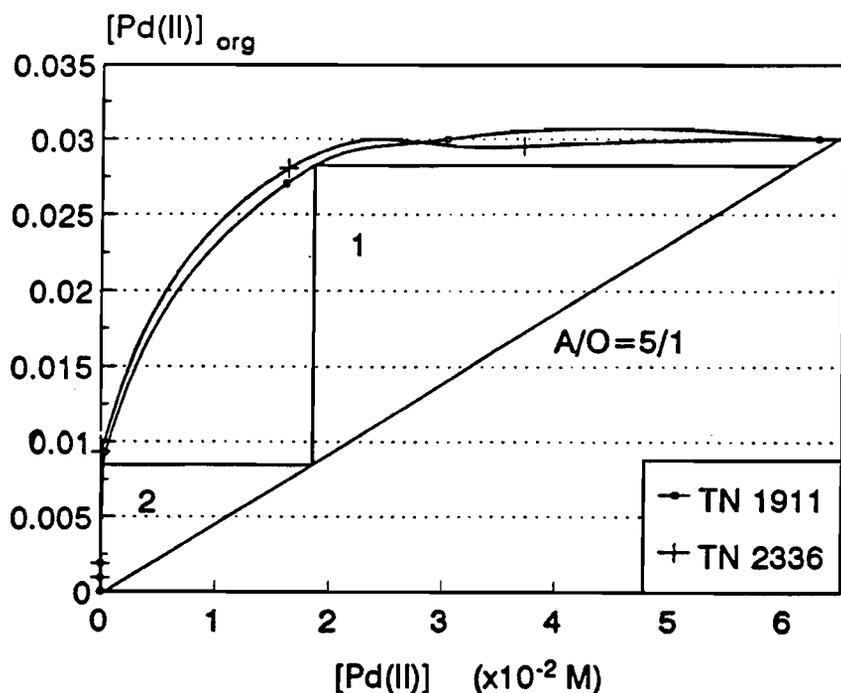
Figure B.3 Equilibrium Pd(II) extraction isotherms and McCabe-Thiele diagram, CT 6 days.
