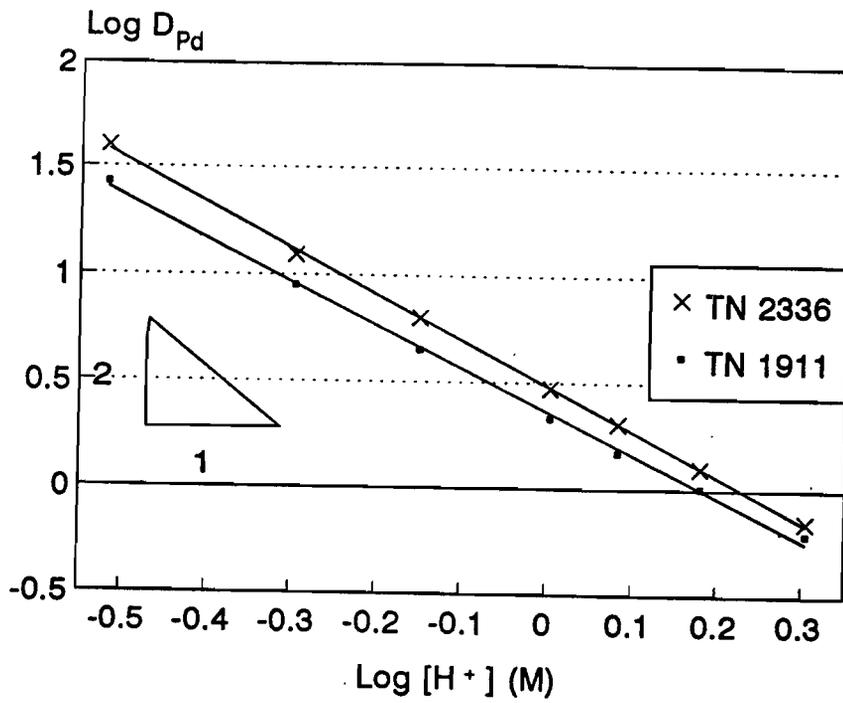
Figure 4.3 Log  $D_{Pd}$  as a function of  $\log [H^+]$  in  $CHCl_3$ .
