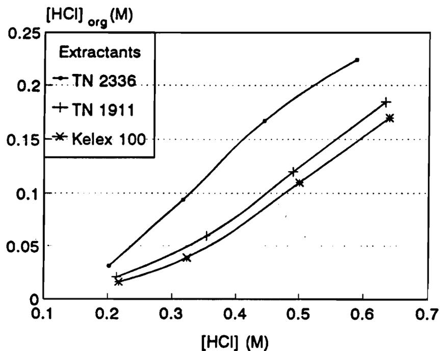
**Figure 3.12** HCl extraction in low acid region  $[\text{Extractant}]_{\text{org}} = 0.50\text{M}$  and Solvesso 150 and Tridecanol were present.
