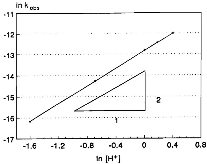
**Figure 6.12** Log-log plot of the observed stripping rate constant,  $\ln k_{obs}$ , versus  $\ln [H^+]$ .
