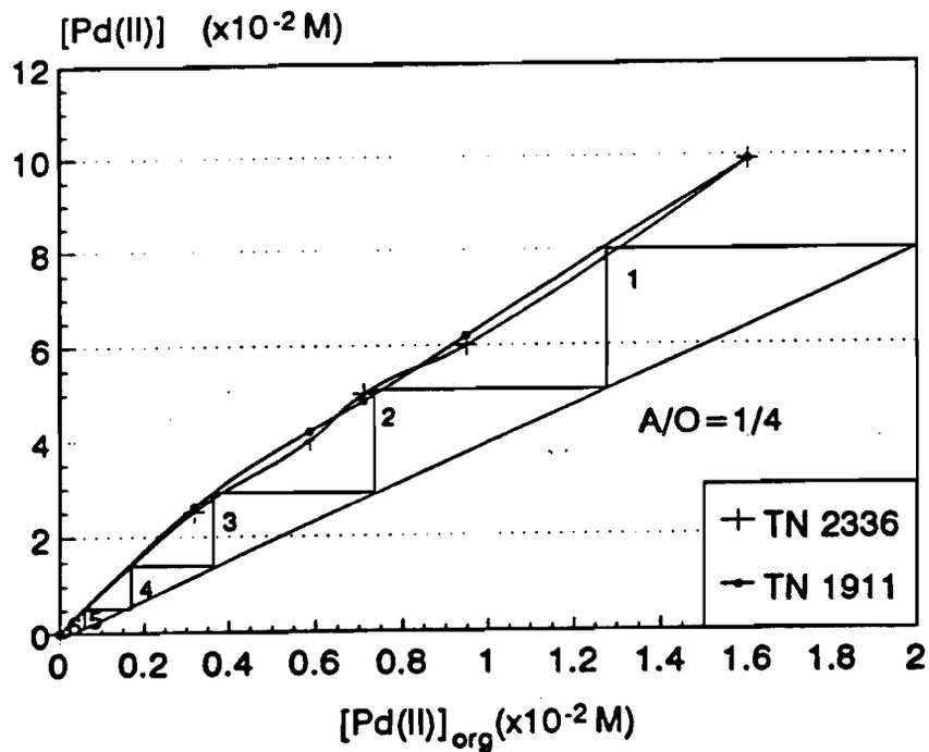
**Figure B.6** Equilibrium palladium stripping isotherms and McCabe-Thiele diagram; stripping agents 6.02M HCl and a mixture 6.02M HCl+2.00M MgCl<sub>2</sub>, CT 6 days.
