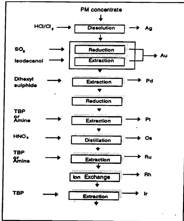
**Figure 2.4** The Lornho refining flowsheet for the separation and recovery of PGM (18).
