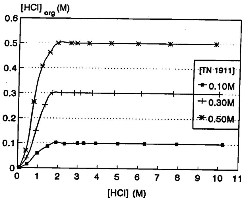
Figure 3.8 HCl distribution in TN 1911 in  $CHCl_3$  solutions.
