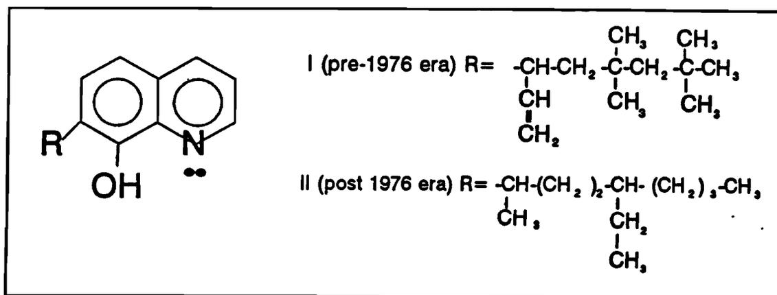
**Figure 2.5** Detailed structure of Kelex 100 (54).
