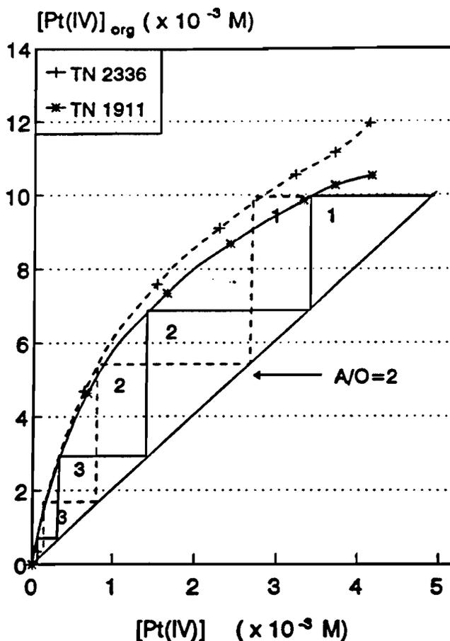
Figure 5.10 Platinum extraction isotherms and McCabe-Thiele diagram.
