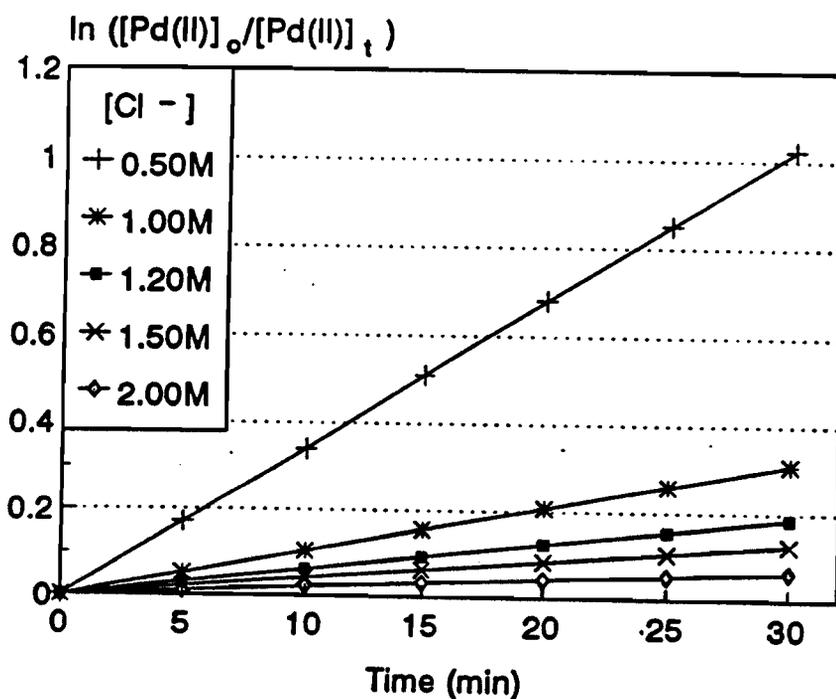
Figure 6.5 First order plots of Pd(II) extraction data at various Cl<sup>-</sup> concentrations.
