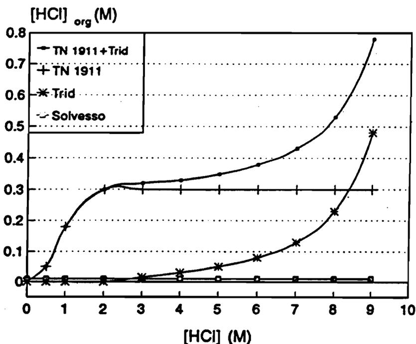
Figure 3.6 HCl distribution in (i) 0.30M TN 1911 + 1.0M Tridecanol, (ii) 0.3M TN 1911, (iii) 1.0M Tridecanol, and (iv) Solvesso 150.
