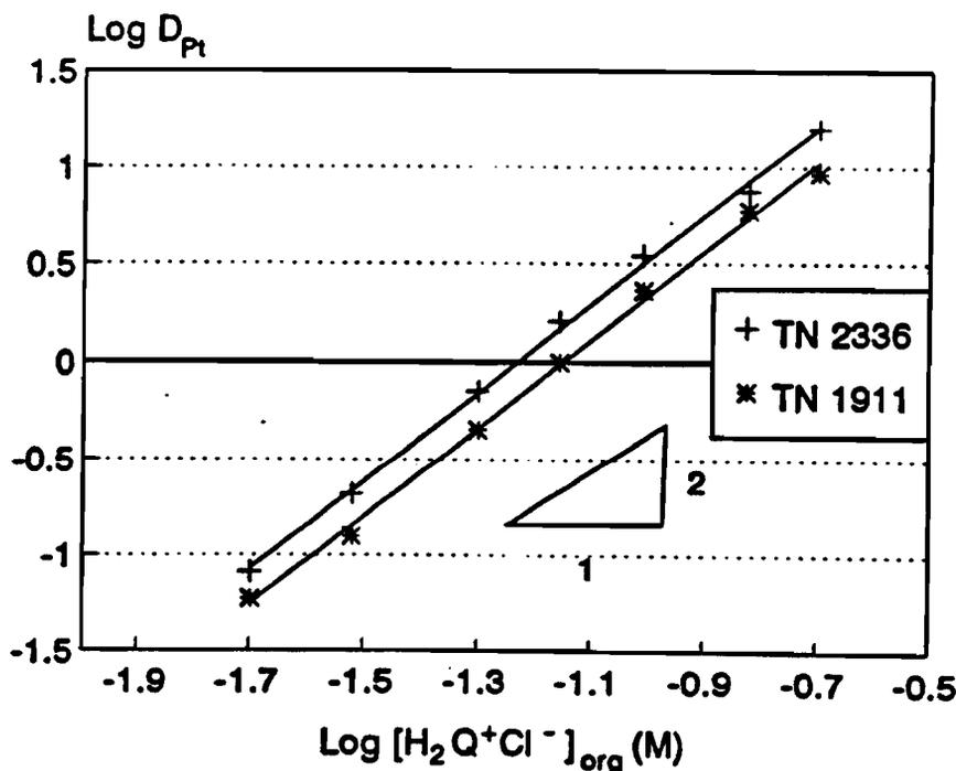
Figure 5.1  $\text{Log } D_{Pt}$  as a function of  $\text{log}[\text{protonated extractant}]_{org}$
