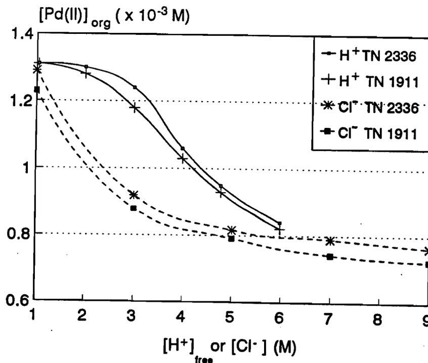
Figure 4.8 Extraction of palladium as a function of H<sup>+</sup> and Cl<sup>-</sup> concentration.
