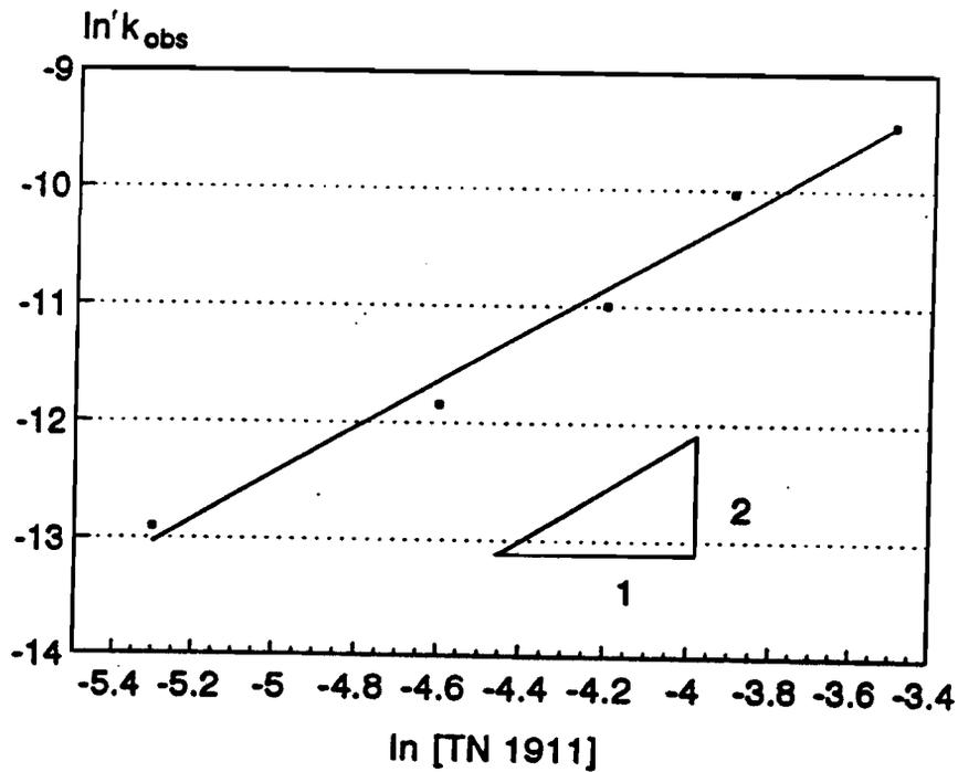
Figure 6.7 Log-log plot of the observed extraction rate constant,  $\ln k_{obs}$ , versus  $\ln [TN\ 1911]$  in  $CHCl_3$ .
