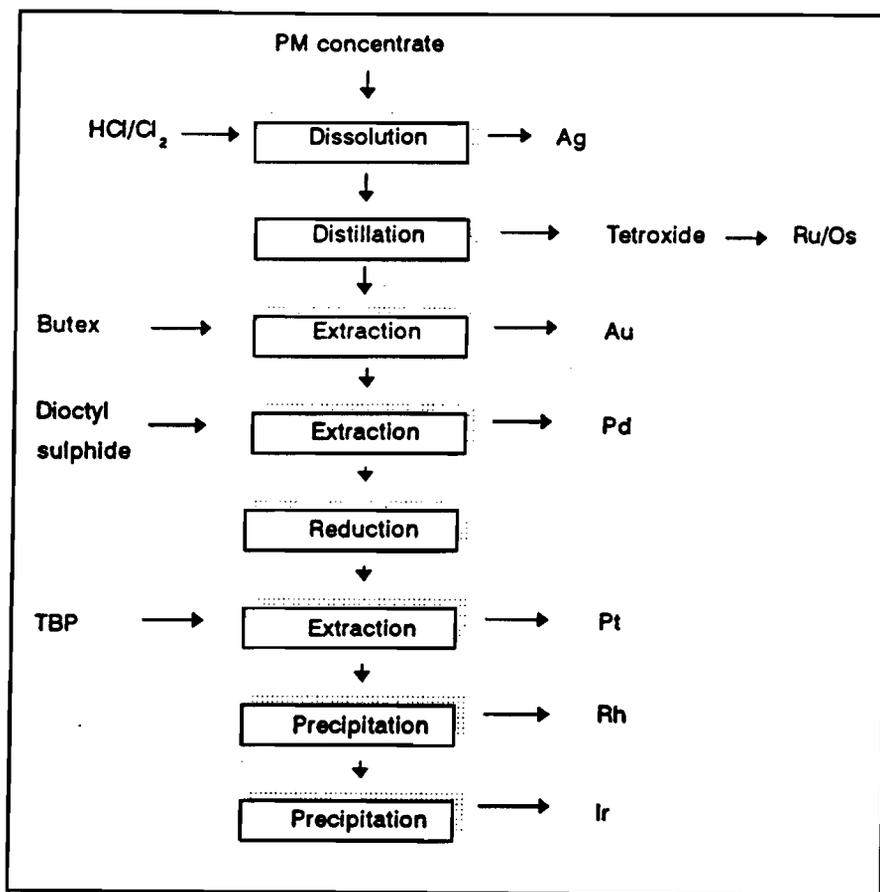
**Figure 2.2** The INCO flowsheet for the separation and recovery of PGM at the Acton plant (5,11).
