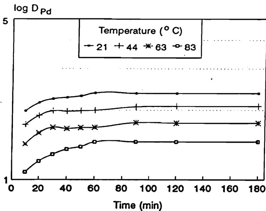
Figure 4.9 Palladium distribution coefficient as a function of temperature and time.
