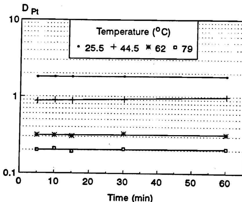
Figure 5.8 Platinum distribution coefficient as a function of temperature and time.
