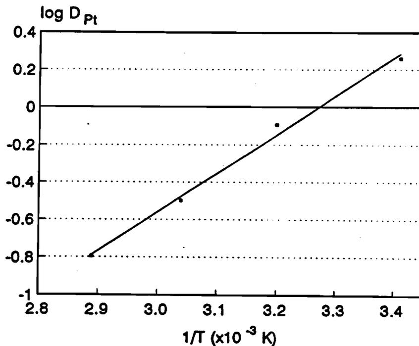
Figure 5.9 Van't Hoff plot for the system Pt(IV)-TN 1911-HCl.
