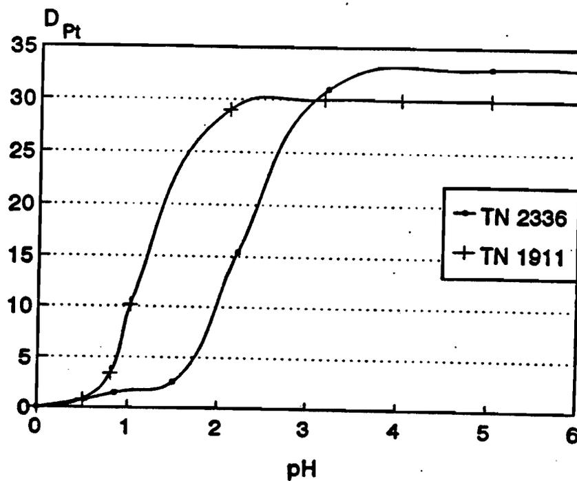
**Figure 5.12** Platinum distribution coefficient as a function of pH.
