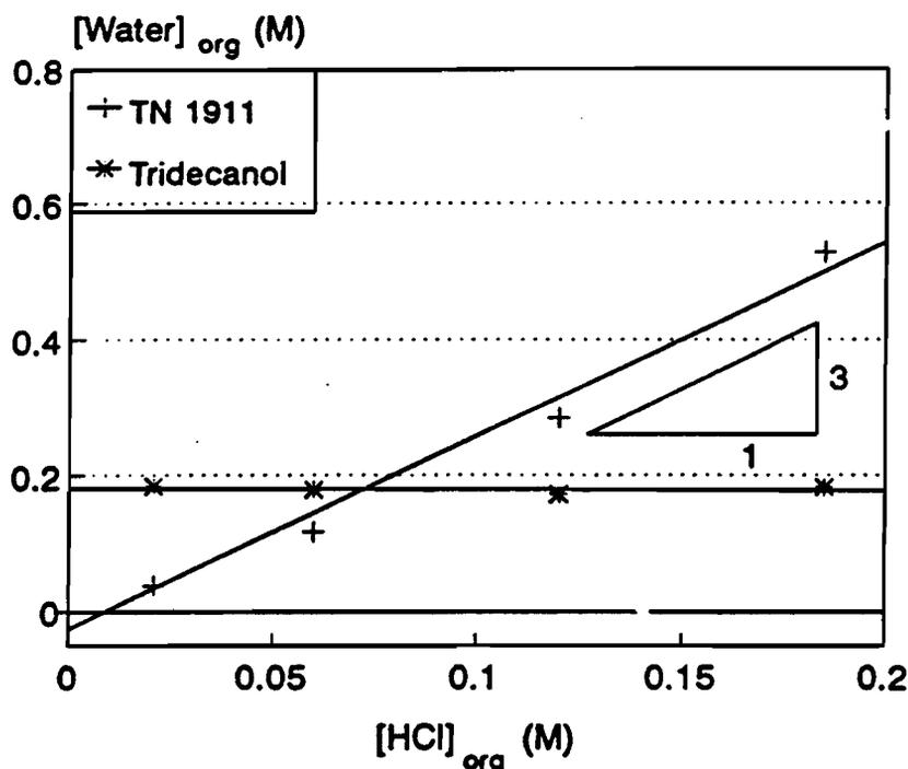
Figure 3.13 Water and acid extracted in low acid region.  $[\text{TN 1911}]_{\text{org}} = 0.50\text{M}$ ,  $[\text{Tridecanol}]_{\text{org}} = 1.58\text{M}$  and Solvesso 150 used as diluent.
