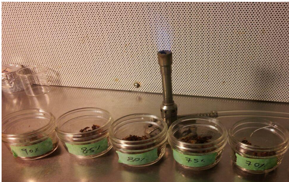
Fig 3.1 Apple pomace samples marked for incubating at different moisture levels (90%, 85%, 80%, 75%, and 70%).
