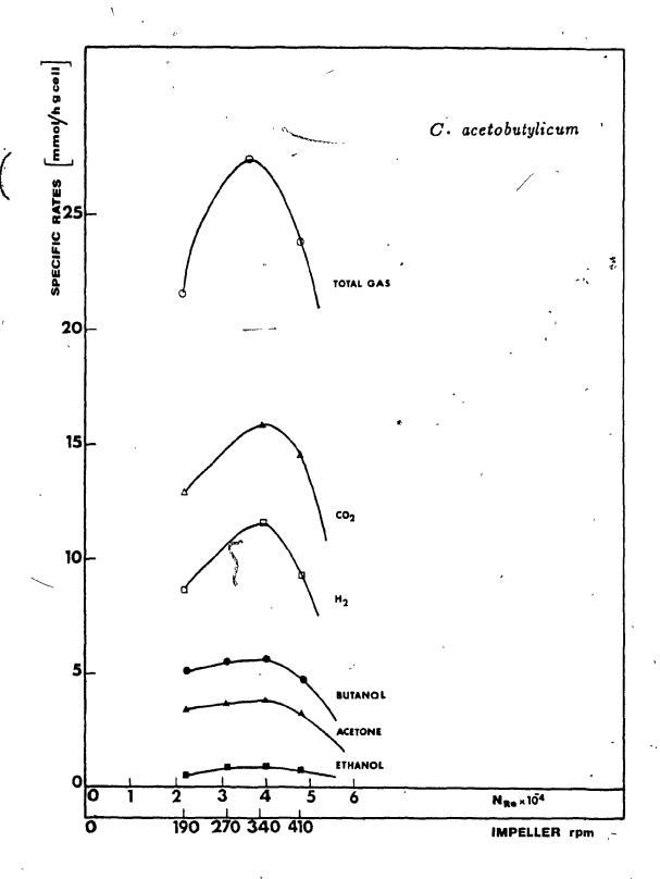
The maximum production rates of the solvents were 5.5 mmole butanol/h·g cell, 3.8 mmole acetone/h·g cell and 0.8 mmole ethanol/h·g cell. These values were obtained at the impeller Reynolds number of 3.93x10<sup>4</sup> (340 rpm).
