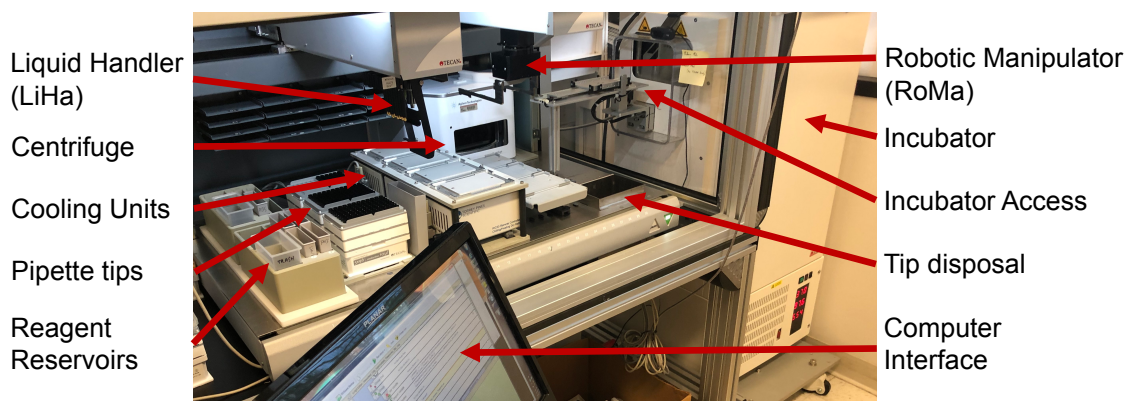
Figure 2.2: Photo of the Immunotron robotic platform built by the Altan-Bonnet lab, with annotations defining its main parts. ( Antigen encoding , [1], SI)
