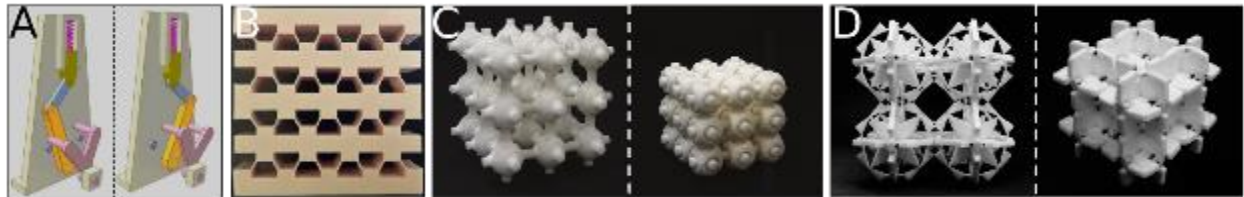
Figure 1-16 Examples of multistable mechanisms and materials; A A bistable mechanism, B A metamaterial made of inclined confined beams undergoing snap-through instability [53], C Perforated shellular structure showing multistability in different directions [23], D A metamaterial made of flexibly hinged links shows multistability in different directions [56].
