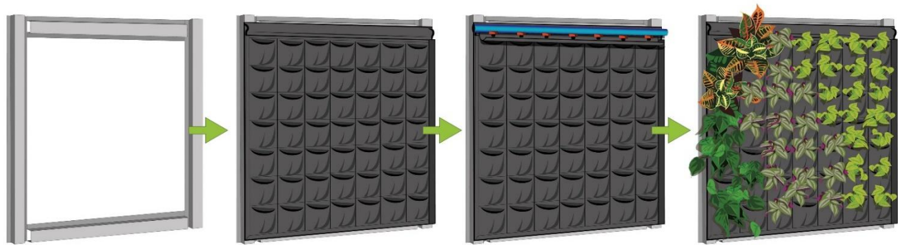
Figure 3.75: Living Wall Installation Process. Living Walls. (n.d.). Retrieved June 22, 2020, from https://www.scotscape.co.uk/services/living-walls
