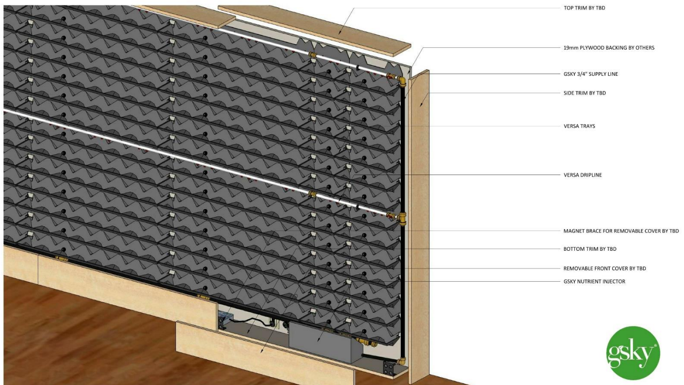
Figure 3.3: Versa Wall Above the Floor/ICU Below Wall VTI-70. Versa Wall CAD & Specs. (2020, March 2). Retrieved from https://gsky.com/versa/cad-specs/
