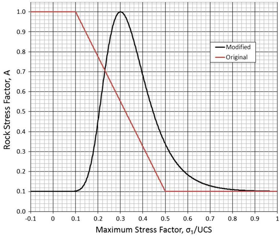
**Figure 2.14** Modified stress factor A, (Mitri et al. 2011)
