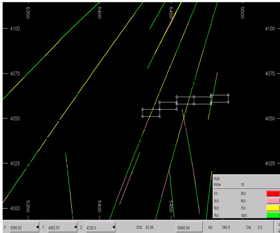
**Figure 4.1** Diamond drills holes plotted and stopes in Datamine
