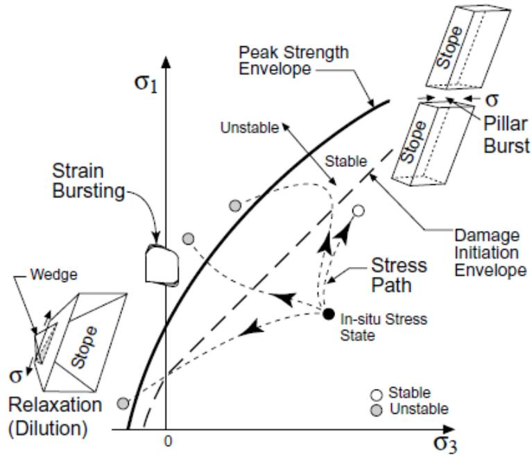
**Figure 2.11** Possible stress path for a stope (Martin et al. 1999)
