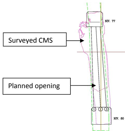
**Figure 6.1** 2D section of an 80 level stope at Lapa Mine
