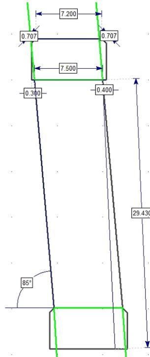
**Figure 6.14** Stope construction geometry
