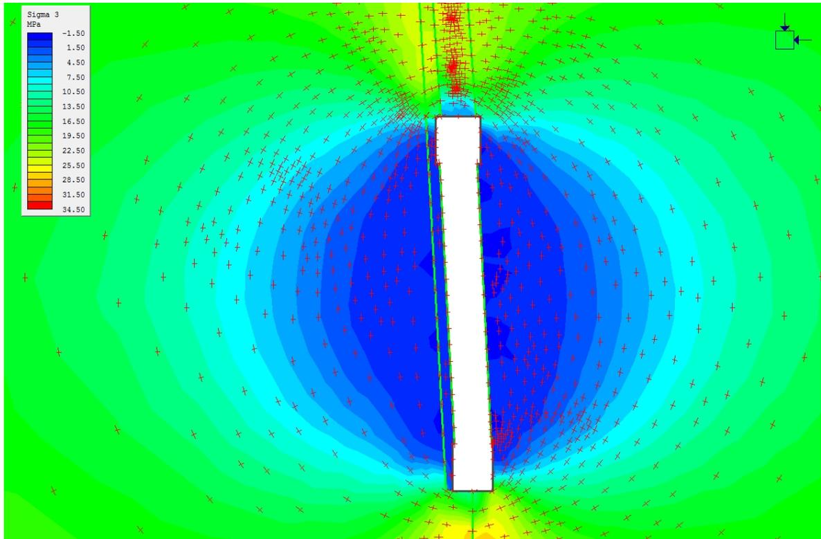
**Figure 5.4** Stress trajectories around the first stope
