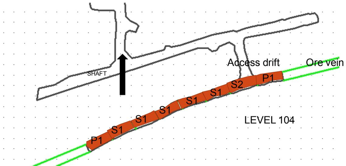
**Figure 6.5** Mining sequence at level 104
