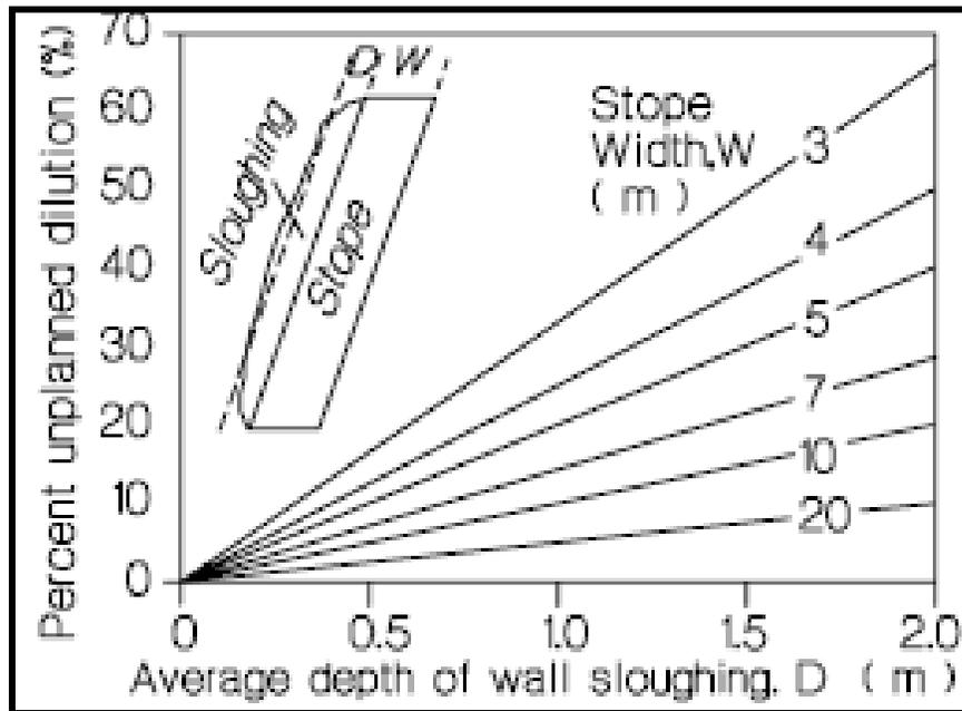
Figure 2.12 Dilution vs sloughing and span (Pakalnis et al. 1995)
