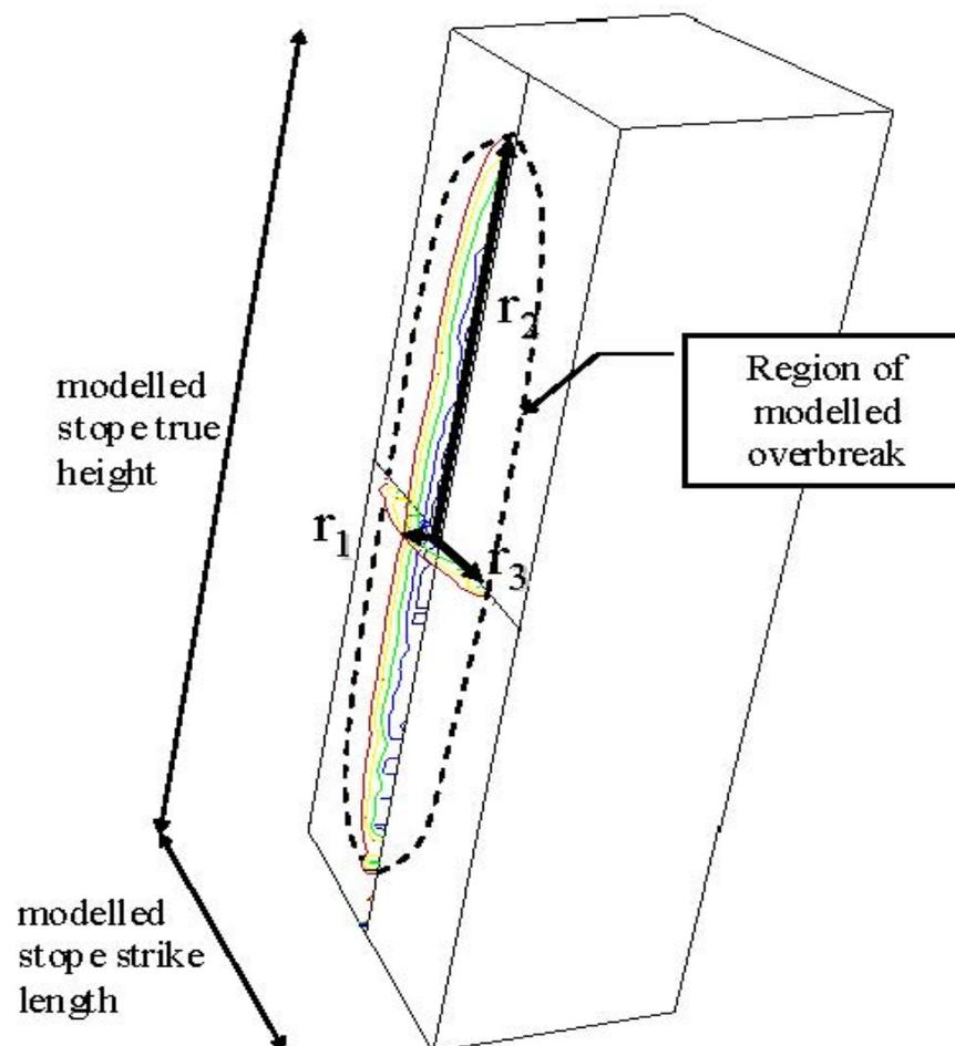
**Figure 2.18** Representation of the half ellipsoid (Henning and Mitri 2007)
