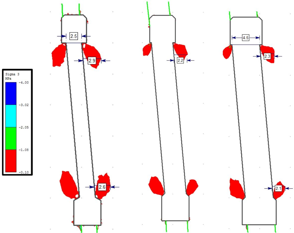
Figure 6.17 Hanging wall tension in stopes with ore width ranging from 2.5m to 4.5m
