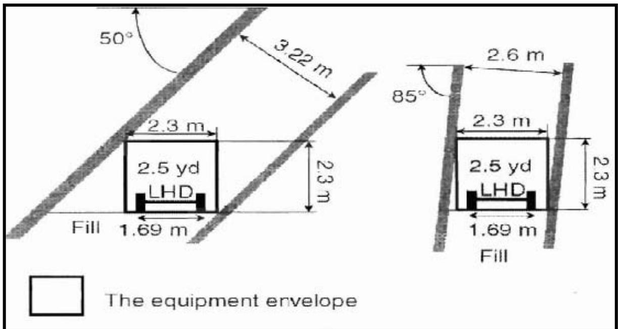
**Figure 2.7** Stope width for differently dipping ore deposits (SME 2001)
