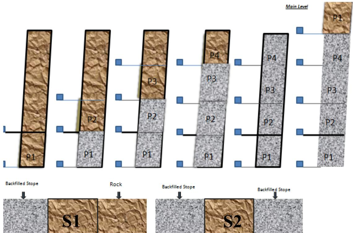
**Figure 2.9** Stope categories within the mining block
