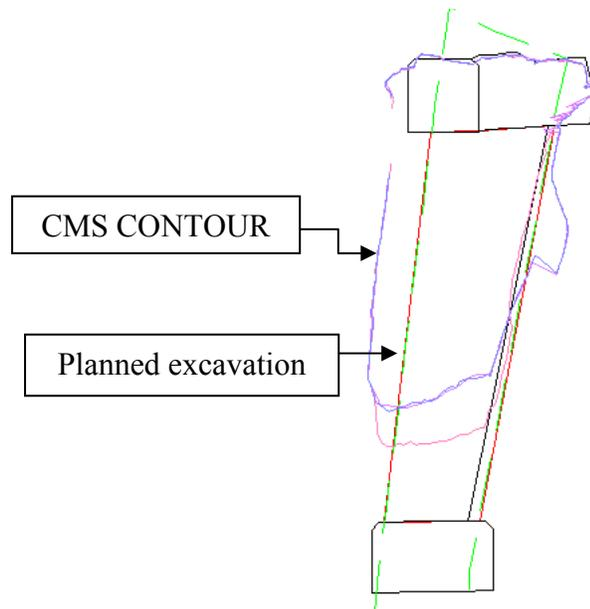
**Figure 2.4** CMS stope survey and planned excavation at Lapa Mine
