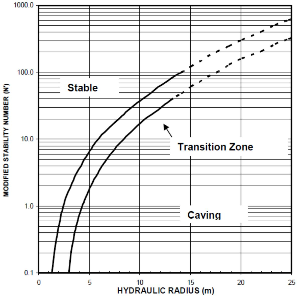
Figure 2.13 Modified stability graph (Potvin et al 2001)
