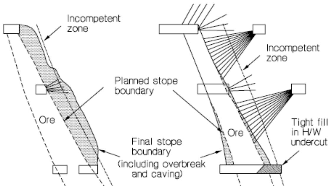
**Figure 2.19** Cable bolting pattern at Helmo mine (after Anderson and Grebenc 1995)
