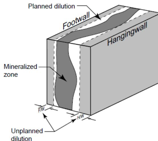
**Figure 2.1** Schematic illustration of different types of dilution
