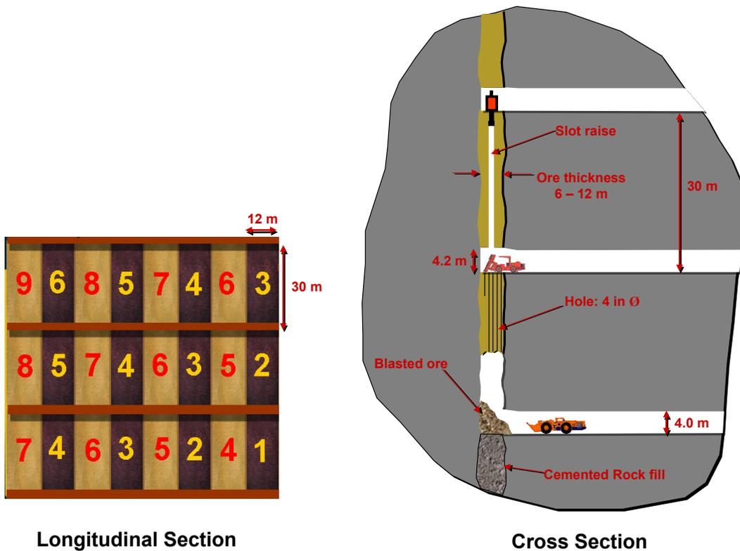
**Figure 3.8** Transversal Primary and Secondary mining method
