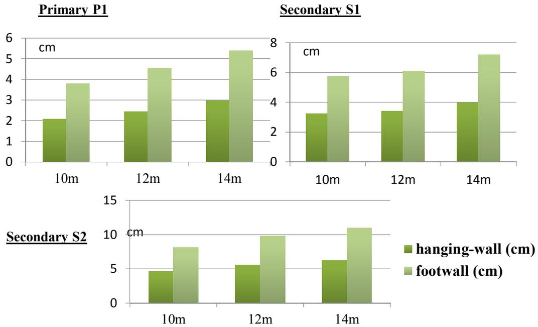
**Figure 6.12** Wall convergence on level 104
