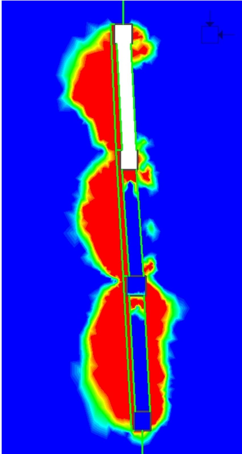
**Figure 5.6** Yield zones around stope with 0.4m undercut
