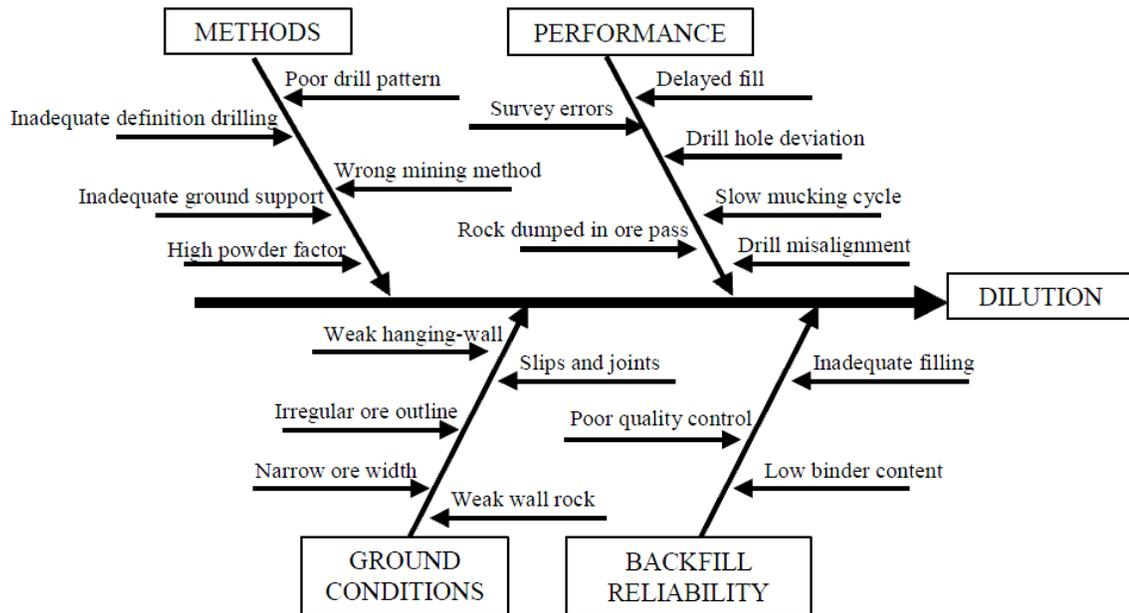
**Figure 2.2** Fishbone chart resuming factors inducing dilution (de la Vergne 2000)
