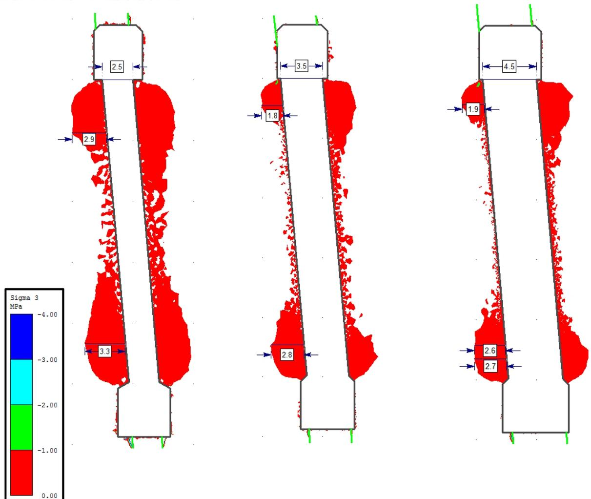
**Figure 6.15** Footwall tension in stopes with ore width ranging from 2.5m to 4.5m
