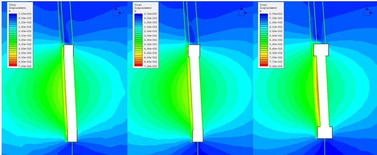
**Figure 5.5** Displacements around the first (lowest) stope
