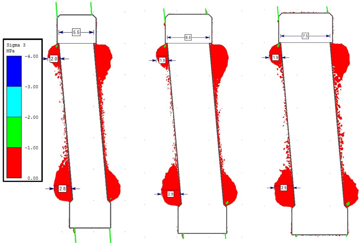
**Figure 6.16** Footwall tension in stopes with ore width ranging from 5.5m to 7.5m
