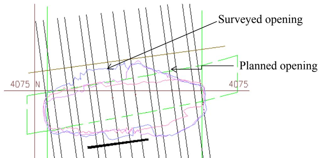
**Figure 2.5** Horizontal cross section at stope mid-height at Lapa Mine
