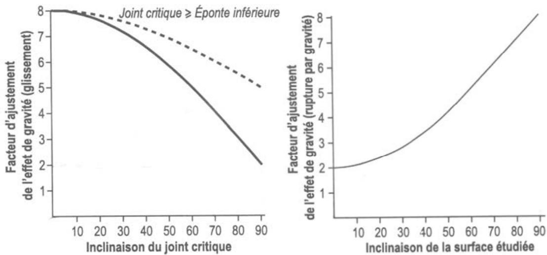
**Figure 2.16** C Factor – case with instability by sliding or gravity instability
