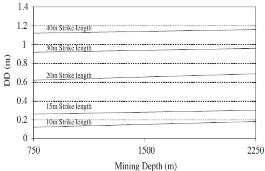
**Figure 6.4** DD vs mining depth and strike length, (Henning 2007)
