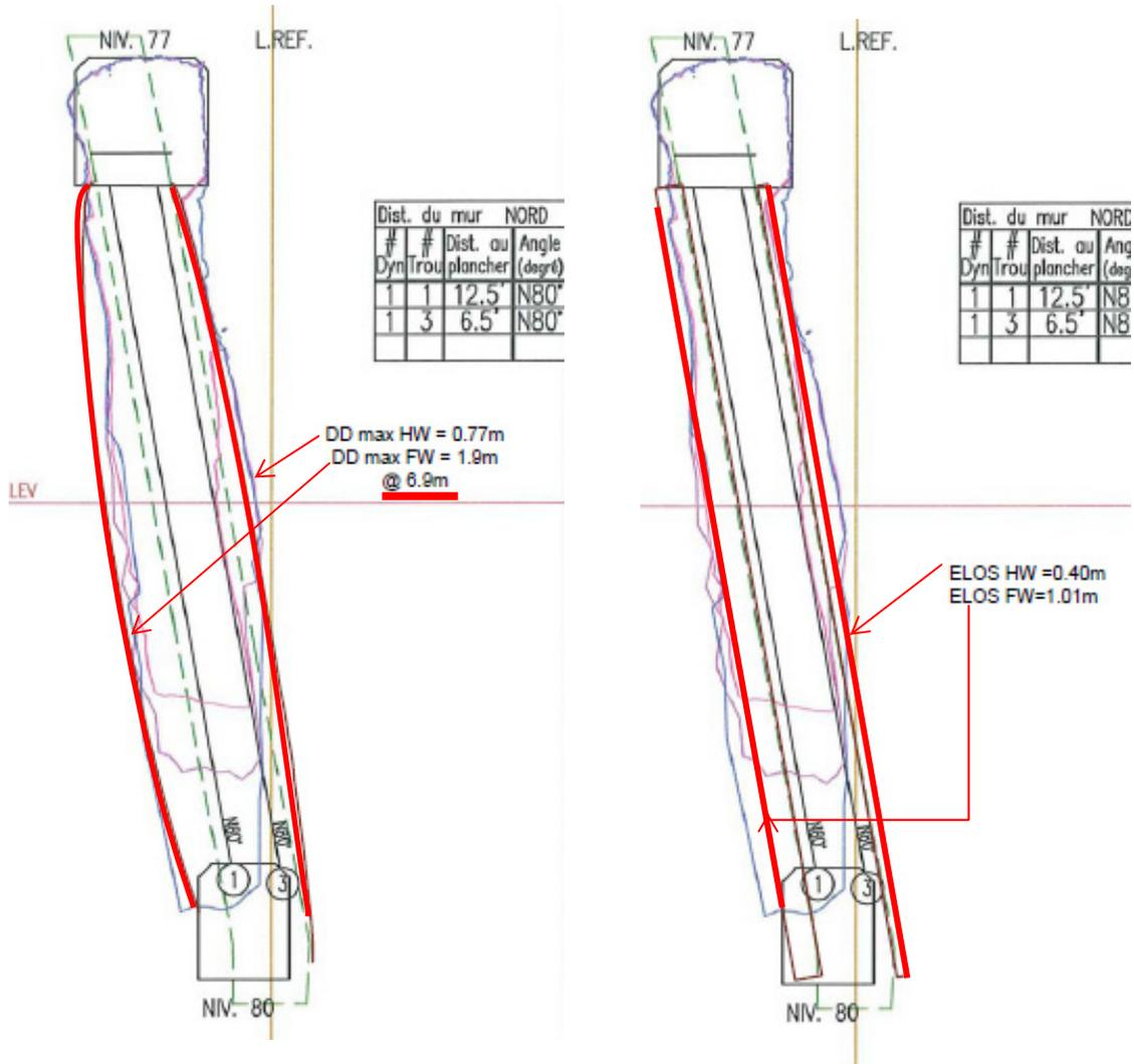
**Figure 4.3** 8049 mid-stope DDmax and ELOS plotted
