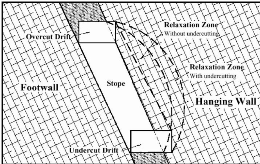
**Figure 2.10** Influence of wall undercutting on stope relaxation (Wang et al. 2002)
