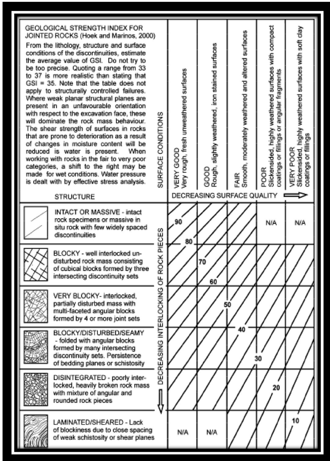
Figure 4.2 Geological strength index GSI classifications (Hoek et al. 2002)
