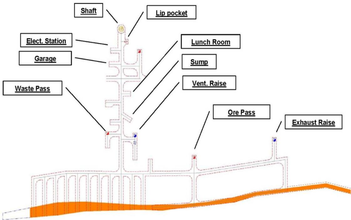
**Figure 3.4** Typical underground services in each level at Lapa, level 800
