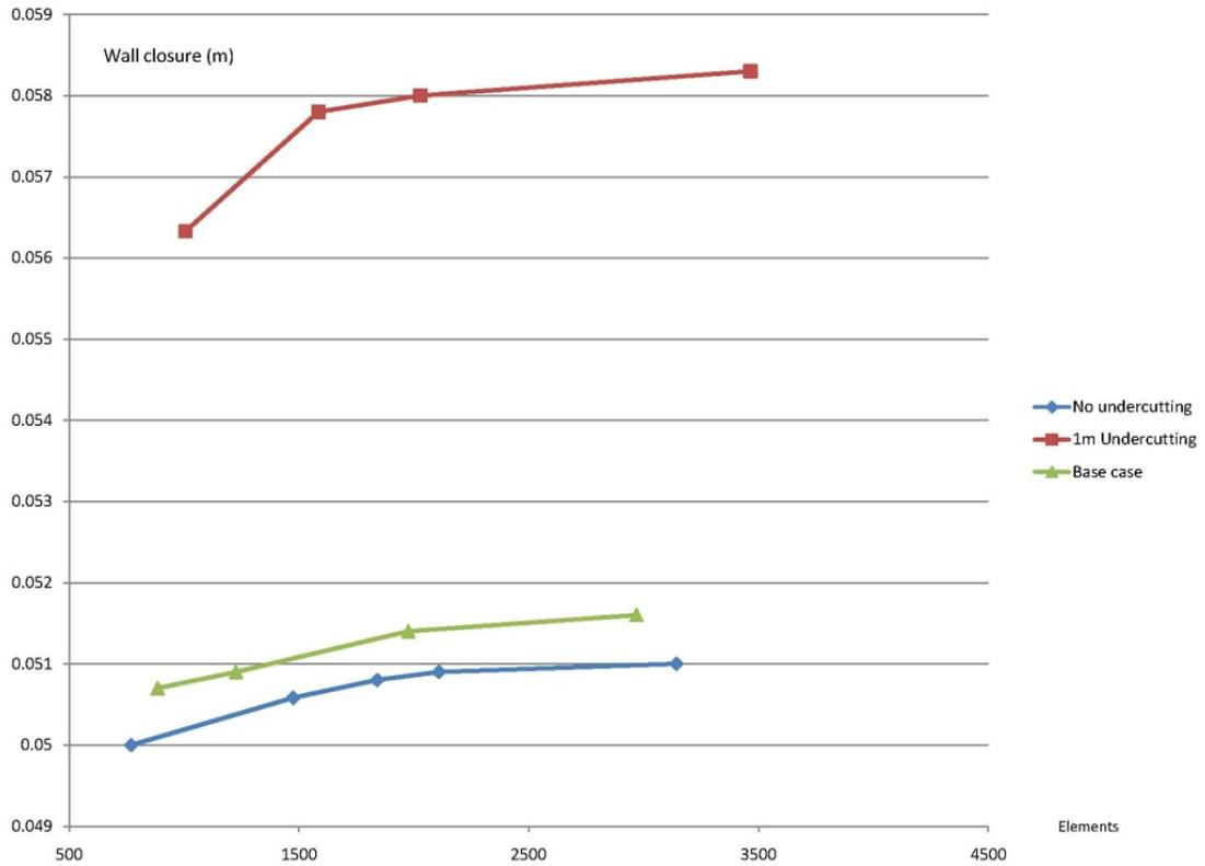
**Figure 5.3** Mesh sensitivity analysis for each of the three models analyzed
