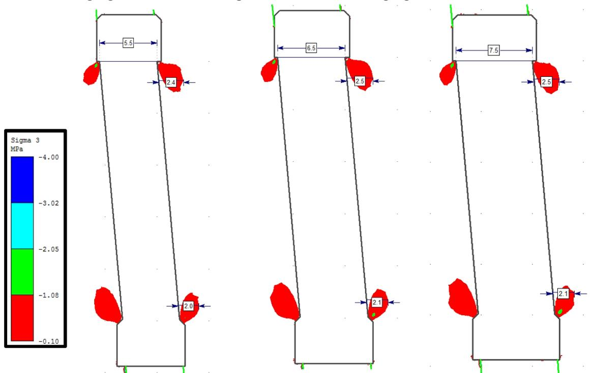
Figure 6.18 Hanging wall tension in stopes with ore width ranging from 5.5m to 7.5m
