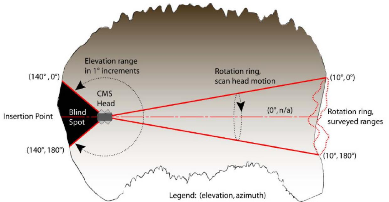
**Figure 2.3** Cavity monitoring system (CMS) in a drift (Optech-CMS advertising)
