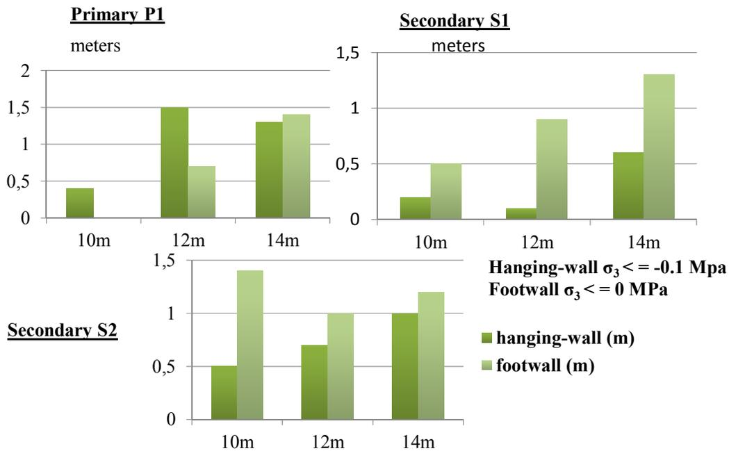
**Figure 6.13** Wall sloughage on level 104
