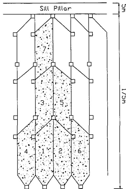
**Figure 4.6** A Longitudinal Section of the Extraction Sequence at Kidd Creek Mine (48)
