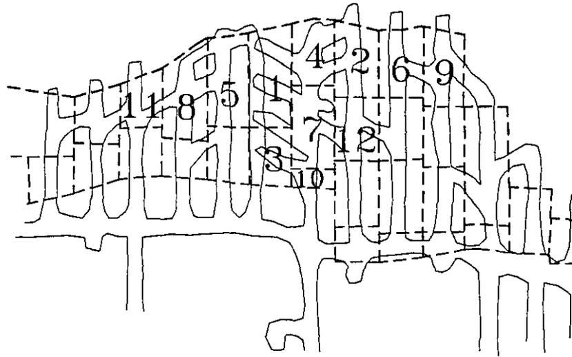
**Figure 4.7** A Plan View of the Single Pass Mining Sequence at Kidd Creek Mine (48)
