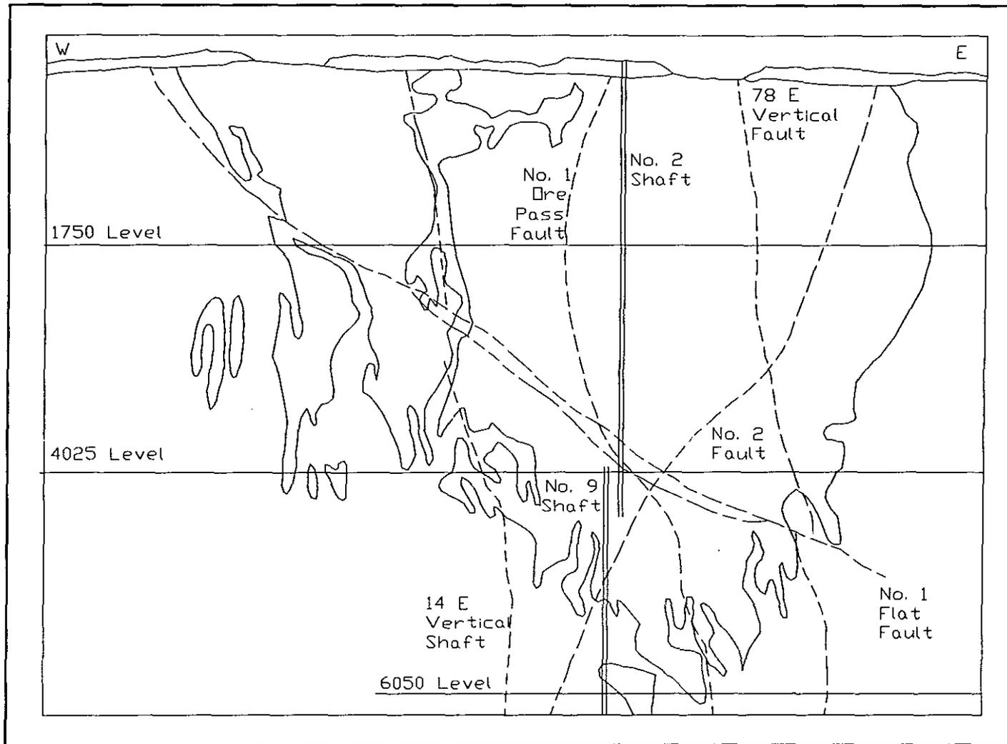
Figure 3.5 A Longitudinal Section Showing Faults at The Falconbridge Mine (9)
