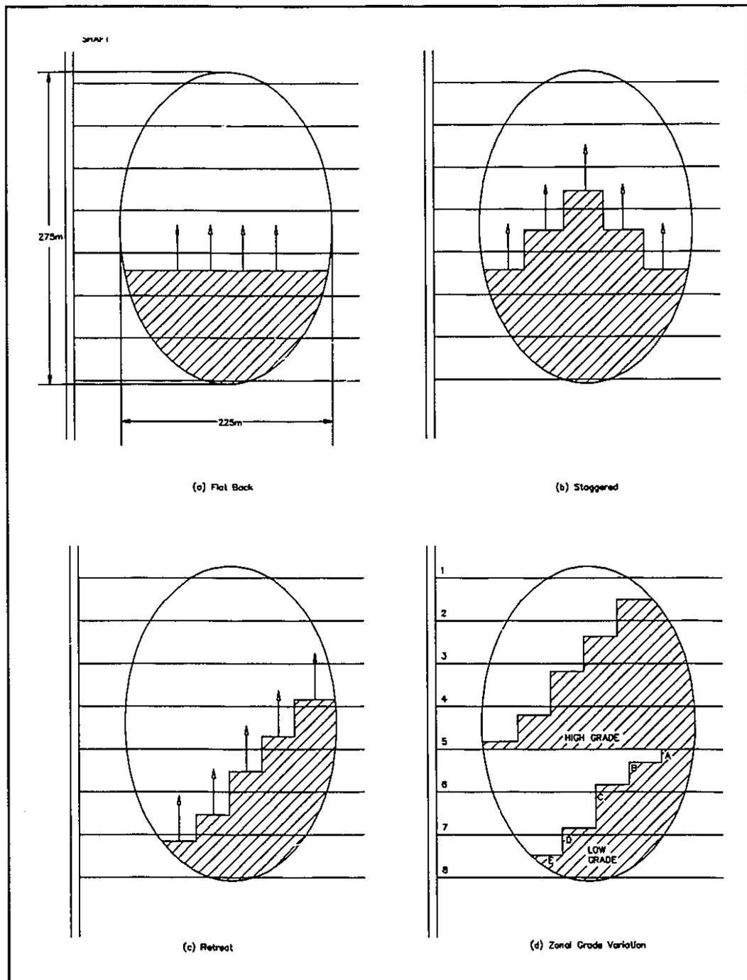
**Figure 3.1** Alternate Stope Extraction Sequences (30)
