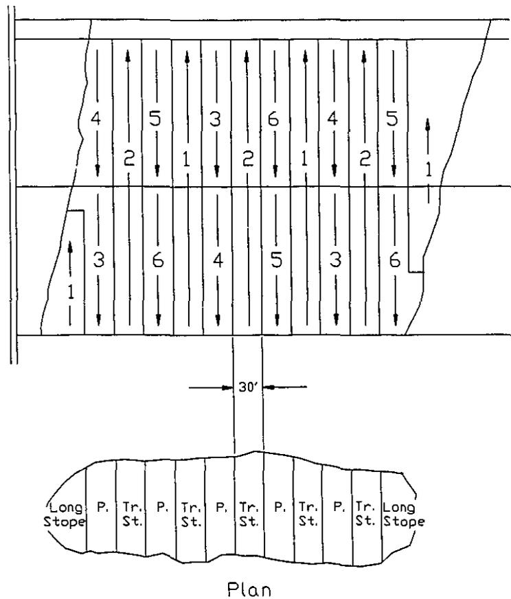
**Figure 4.3 A Mining Sequence for Wide Ore (30)**
