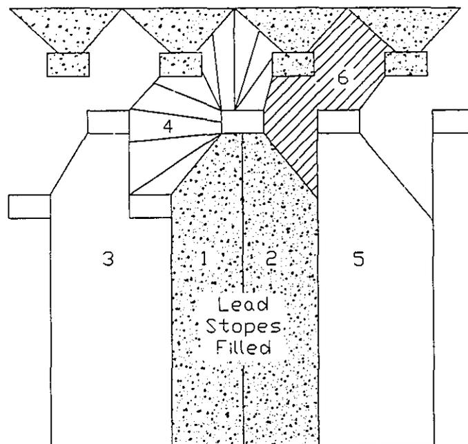
**Figure 4.9 Sill Pillar Removal at Kidd Creek Mine (48)**
