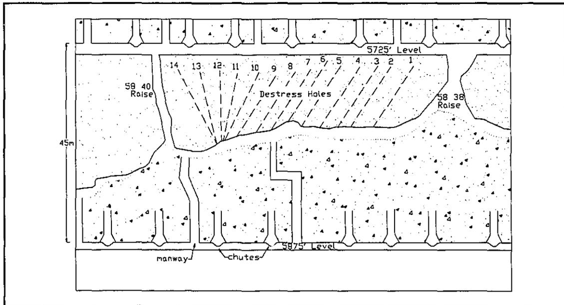
Figure 3.10 A Destress Blast in a Sill Pillar at the Macassa Mine (40)
