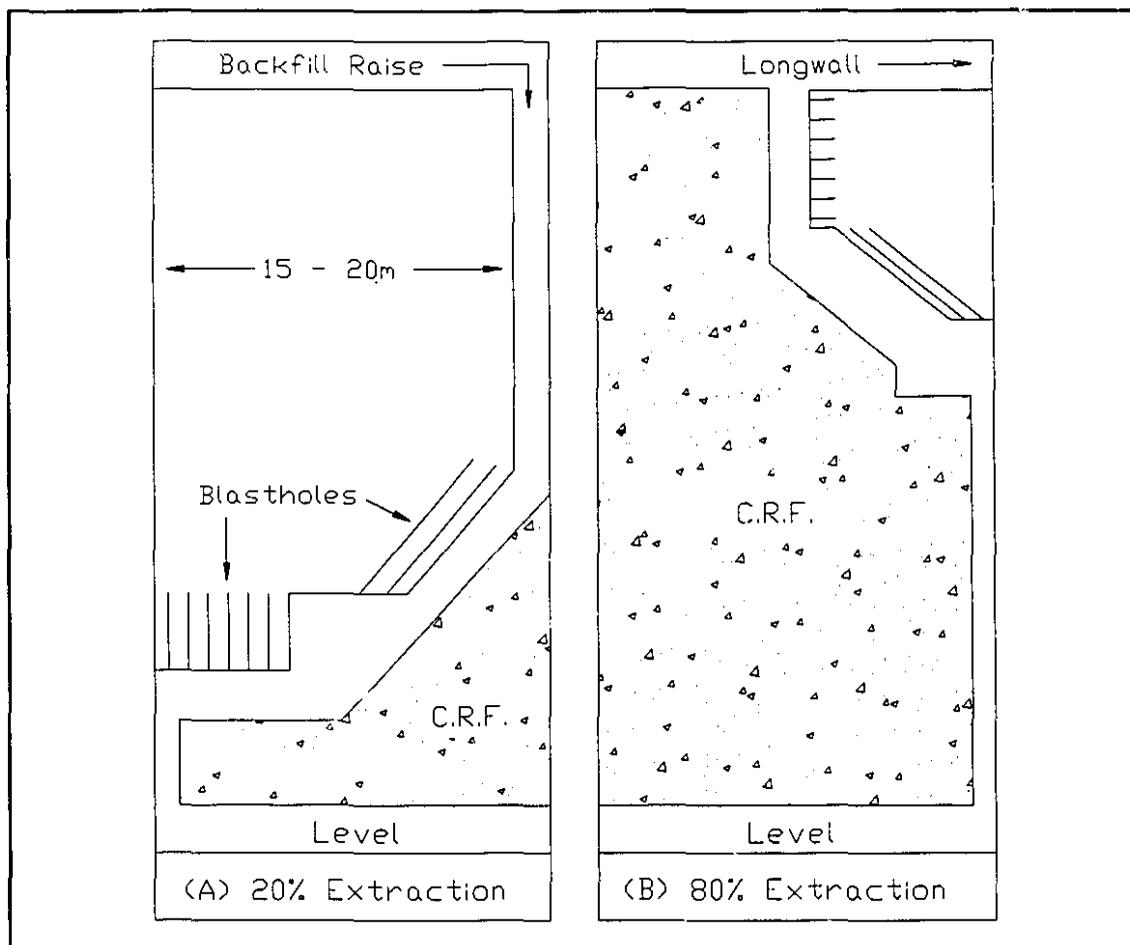
**Figure 3.11** The Rill Mining System Developed for the Macassa Mine (42)
