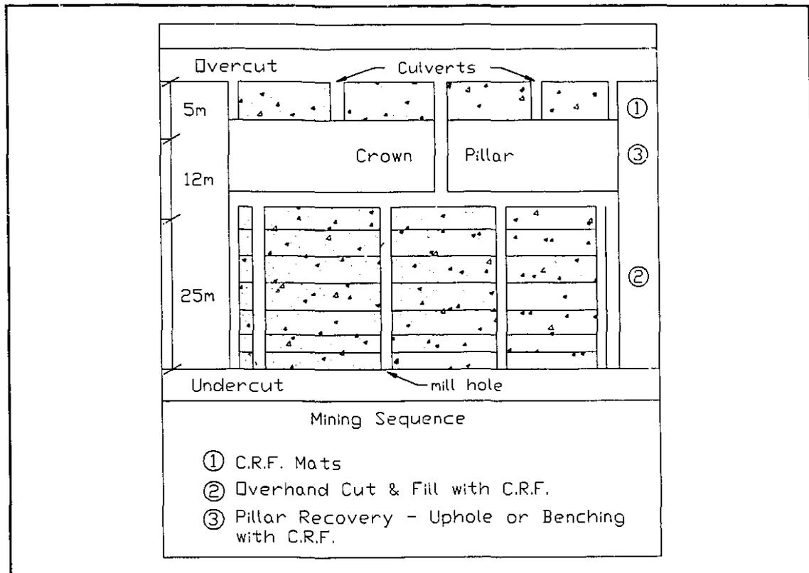
Figure 3.12 A Longitudinal Section of the Trial Mining Method at the Macassa Mine (42)
