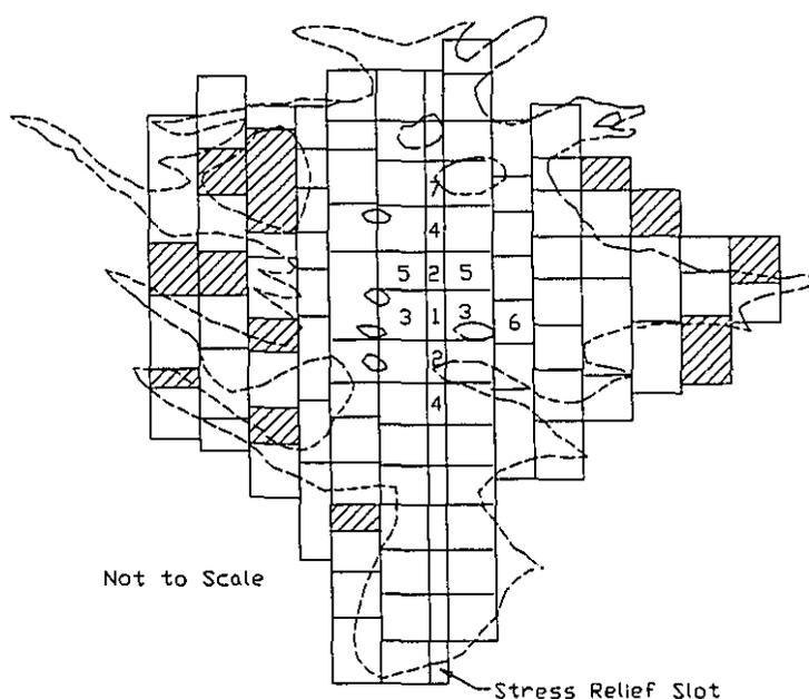
**Figure 4.11** Creating a Destress Slot at the Creighton Mine
