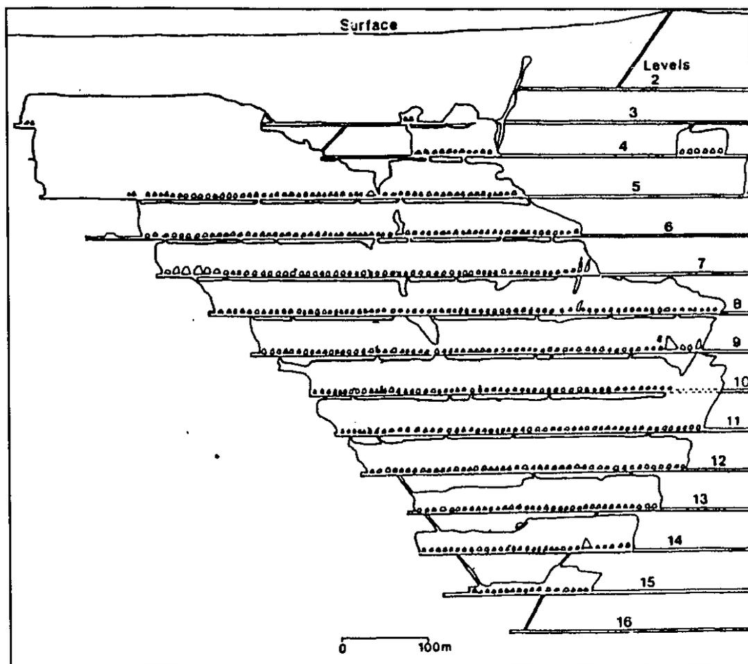
**Figure 3.7** A Longitudinal Section of the F Zone at the Campbell Red Lake Mine
