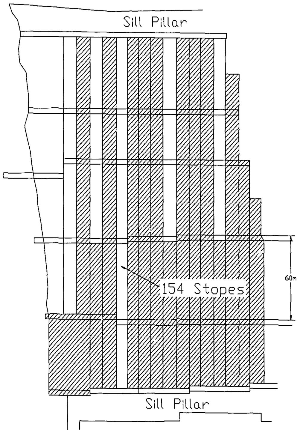
Figure 4.5 The Tertiary Mining Sequence from the Lockerby Mine
