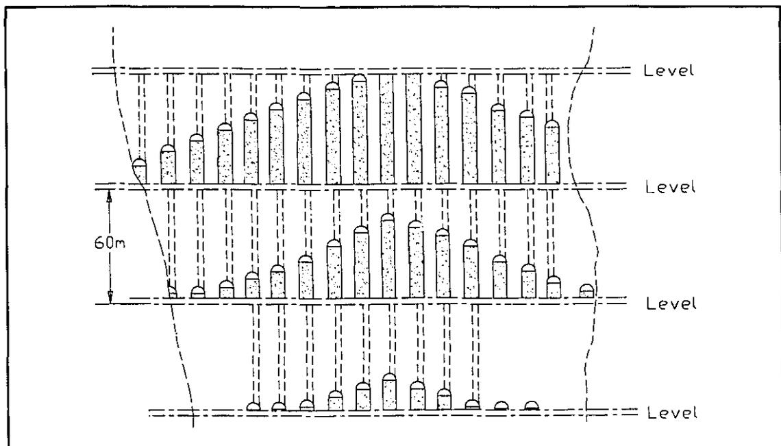
**Figure 3.14 A Conventional Transverse Mining Layout Using a Domed Sequence (43)**
