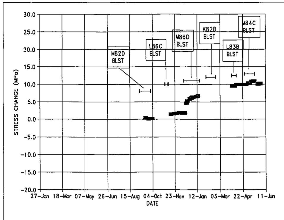
**Figure 7.11 Stress Cell: M84D, 7 Level Undercut**
