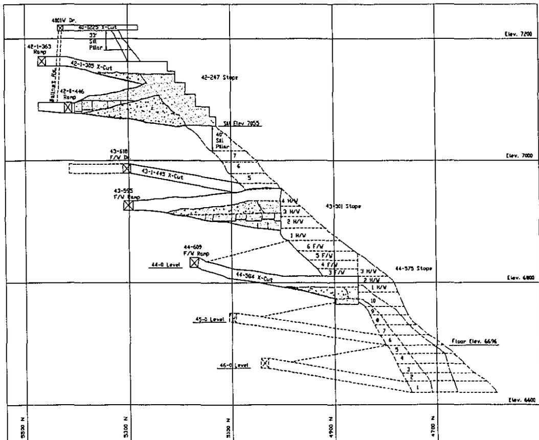
Figure 4.1 A Vertical Pillar at the Onaping Mine
