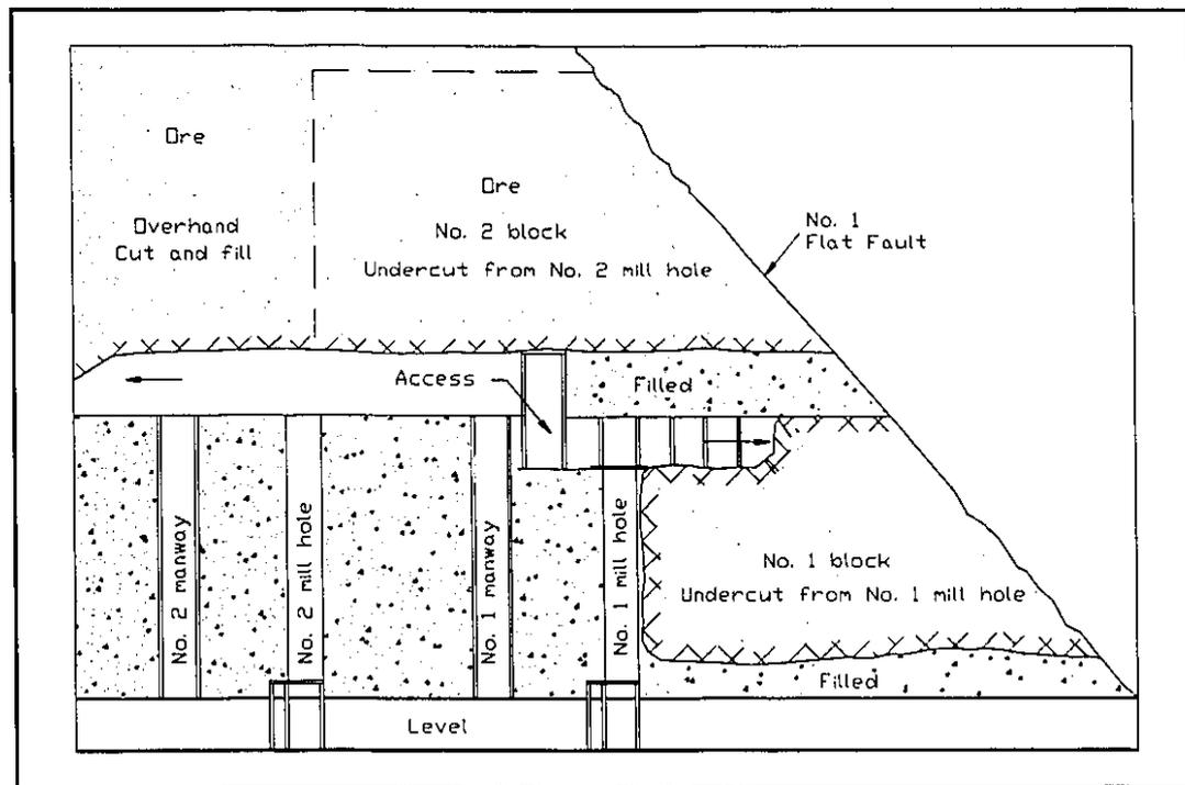
**Figure 3.6 Underhand and Overhand Methods used below a Flat Fault (33)**
