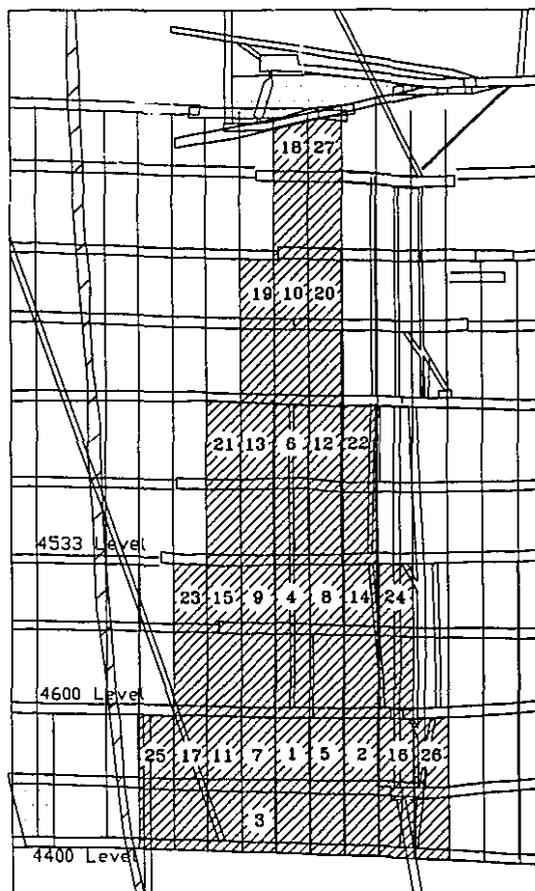
**Figure 5.8** Golden Giant Mine, Sequence in Block 3
