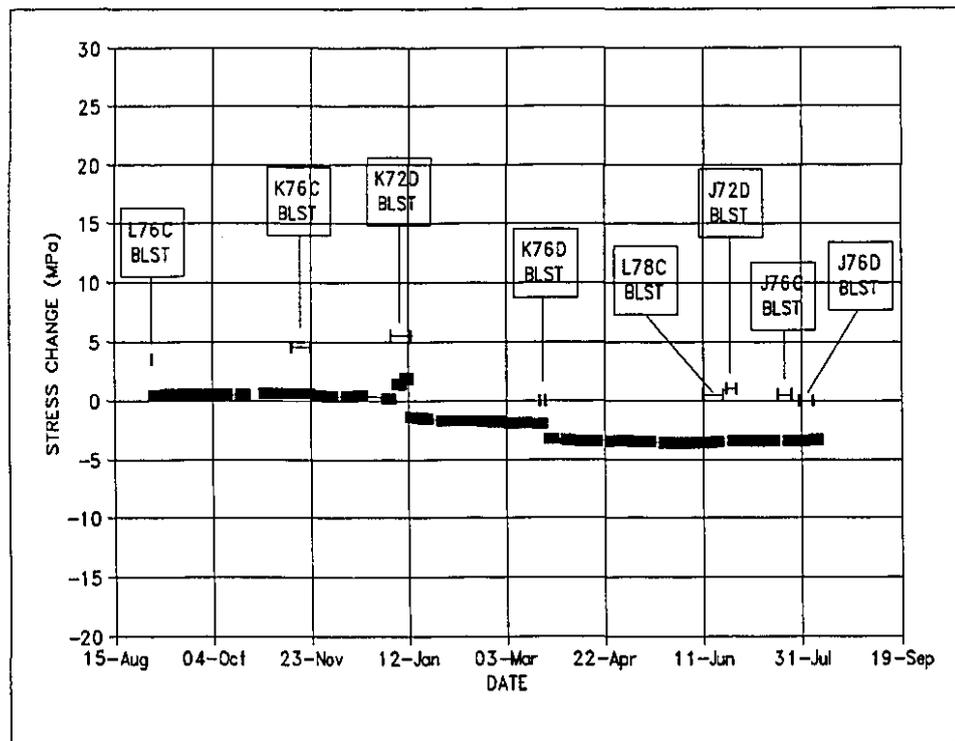
**Figure 7.4 Stress Cell: K72C-FW-AS, 7C Haulage**
