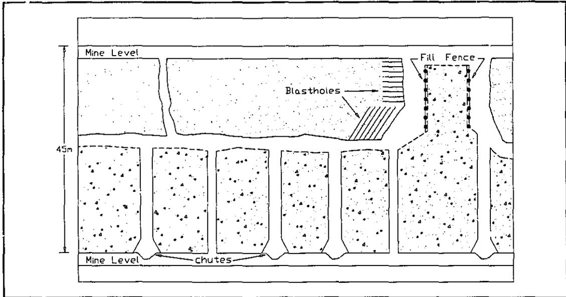
Figure 3.9 A Rill System of Sill Pillar Recovery at the Macassa Mine (40)
