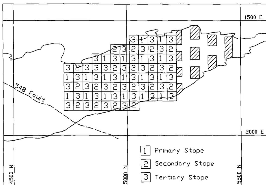
**Figure 4.13** The Eggcrate Sequence at Mount Isa Mines (After Alexander and Fabjanczyk 1981)
