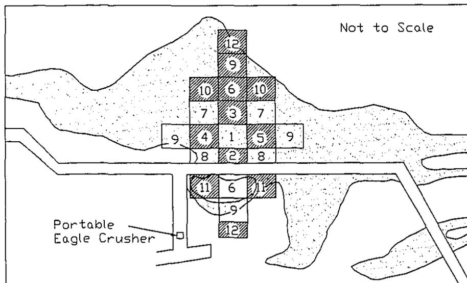
**Figure 4.12** The Mining Sequence for Deep Ore at Creighton Mine
