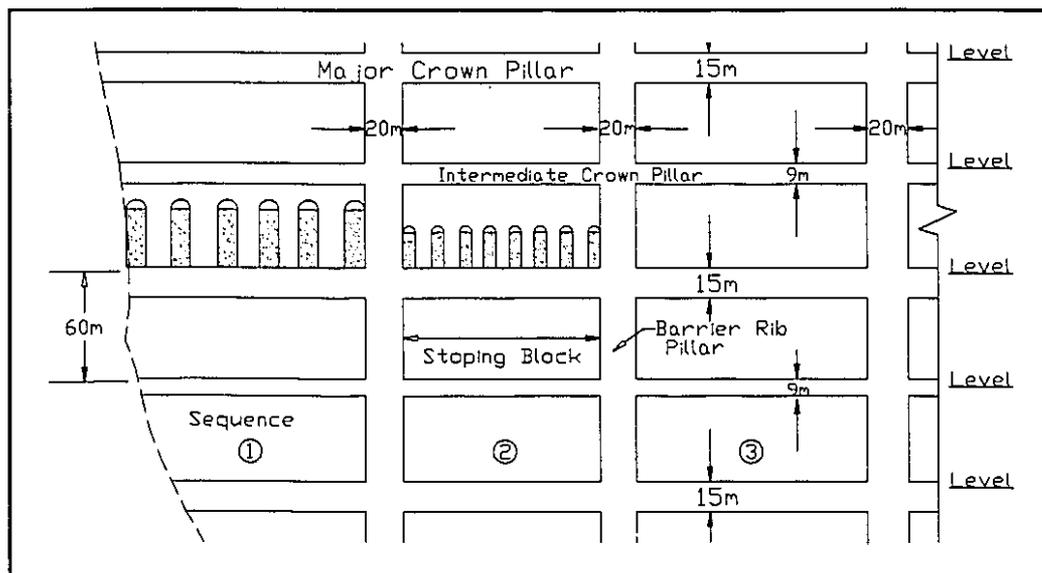
**Figure 3.13** An Historical Longitudinal Layout from the Frood Mine (43)
