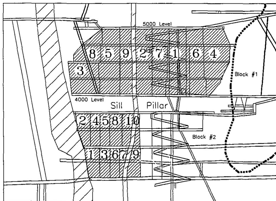
Figure 5.7 Golden Giant Mine, Sequence in Blocks 1 and 2
