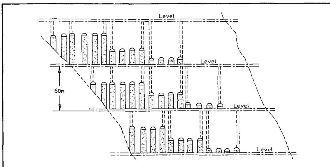
**Figure 3.15 A Mechanized Transverse Mining Sequence (43)**
