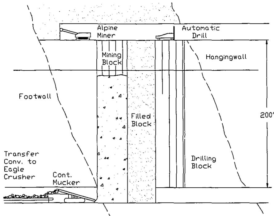
**Figure 4.10** Excavating the Drili Access Using an Alpine Miner
