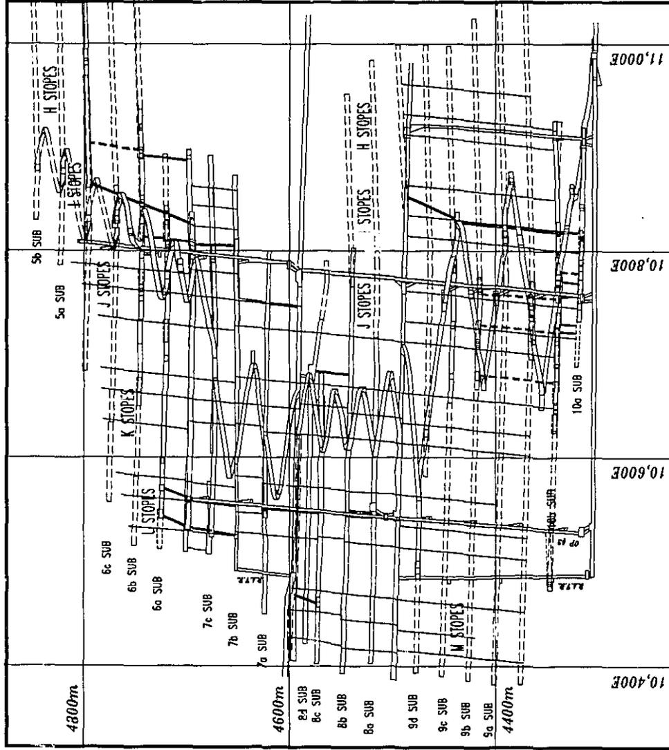
Figure 5.11 A Longitudinal Section of the Present Mining Area
