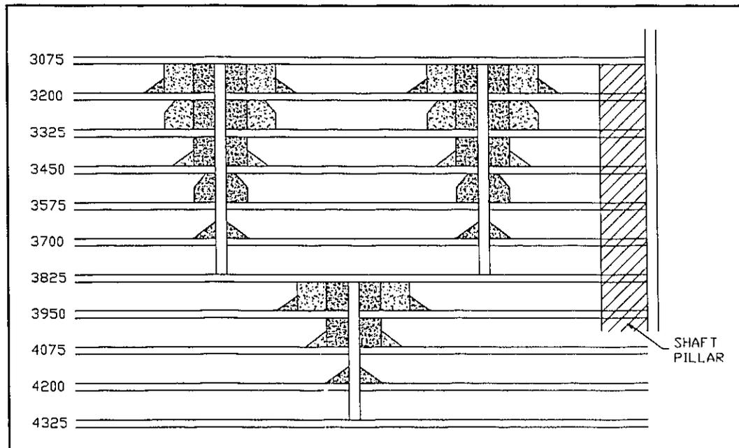
**Figure 3.4** The Steep Rill Mining System at the Lakeshore Mine (31)
