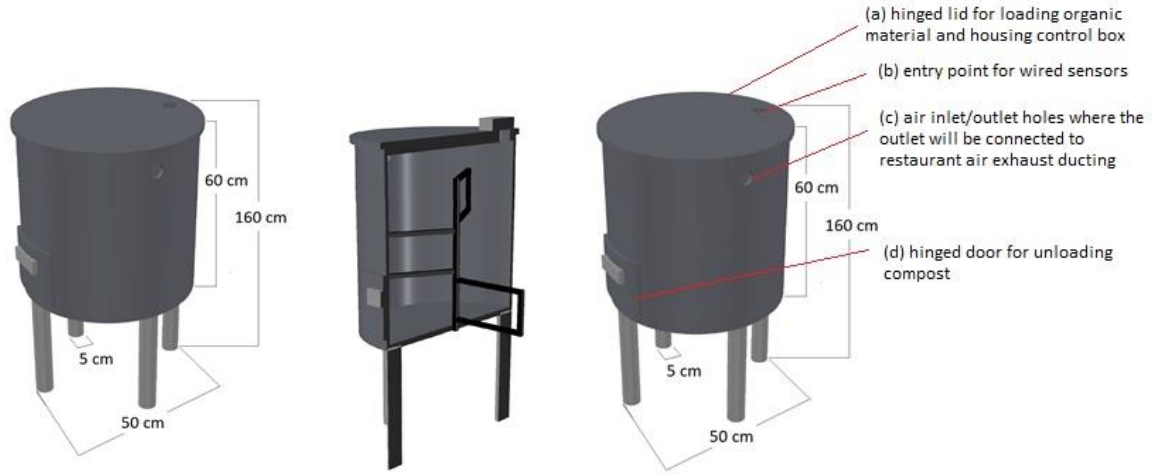
Figure 8: Section and dimensioned schematic of prototype composter
