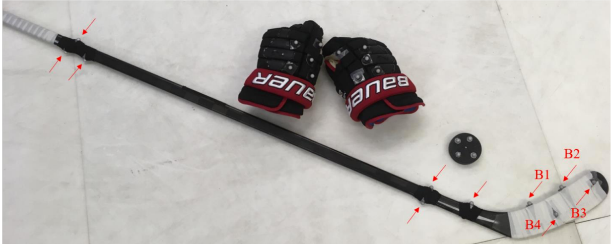
Figure 7. Reflective marker placement on gloves, stick and puck. Markers on the stick are indicated by the red arrows (Denroche, 2020). IMU sensors were placed within an opening in the padding on each glove's thumb.
