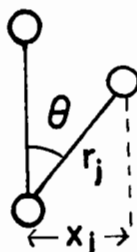
FIG. 2.2 SPECIAL MODE OF VIBRATION: BENDING
