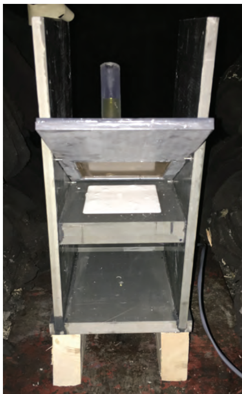
Figure 2.5: Normally incident detonation experiment using the 0.25-mm-thick-slapper with the test explosive cavity filled with a mixture of gelled NM and 10% GMBs.
