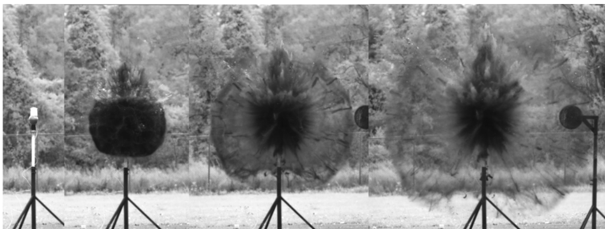
Figure 4.5: Single video frames taken during the explosive dispersal of S110 steel shot particles. Charge diameter is 12.7 cm dia., mass of steel is 4130 g, mass of C-4 is 75 g, giving M/C = 55.1 . Pictures shown were taken at times of 0, 2, 4, and 6 ms after detonation of the charge.
