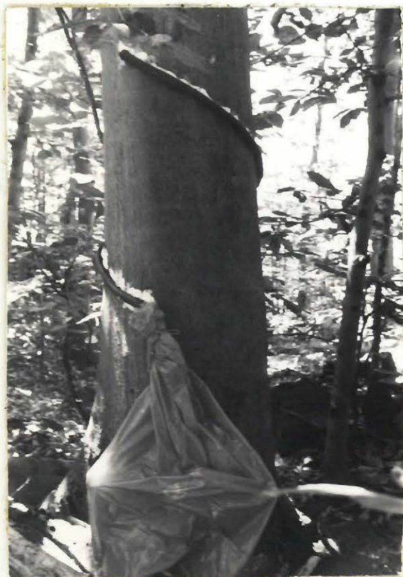
Illustration 7. Measuring stemflow on beech tree.
