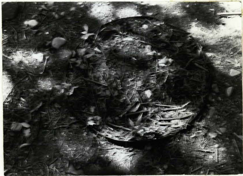
Illustration 10. Evapotranspirometer tank at forest floor.
