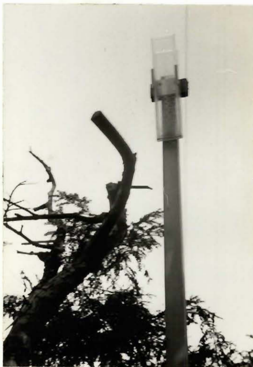
Illustration 5. Rain gauge mounted above the forest.
