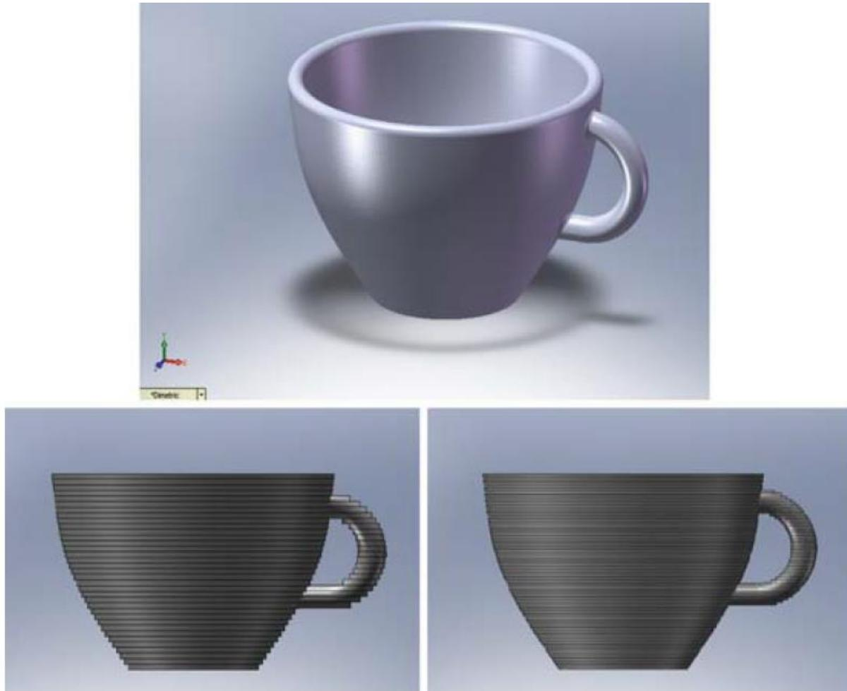
Figure 2.9: Example of the effect of layer thickness on final build resolution [2.30].
